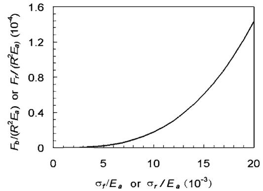
FIG. 3. Relationships between the normalized bifurcation force  $F_b/(R^2 E_a)$  and the normalized forward transformation stress  $\sigma_f/E_a$  and between the normalized return force  $F_r/(R^2 E_a)$  and the normalized reverse transformation stress  $\sigma_r/E_a$  for  $\nu_a=0.3$  under small deformation condition.
