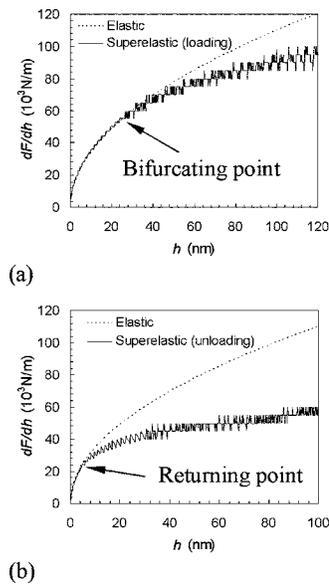
FIG. 4. (a) Determination of the bifurcating point from the elastic slope and superelastic slope curves for the loading process, and (b) determination of the returning point from the elastic slope and superelastic slope curves for the unloading process.
