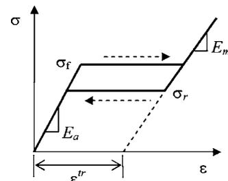
FIG. 1. An idealized superelastic model under uniaxial loading.
