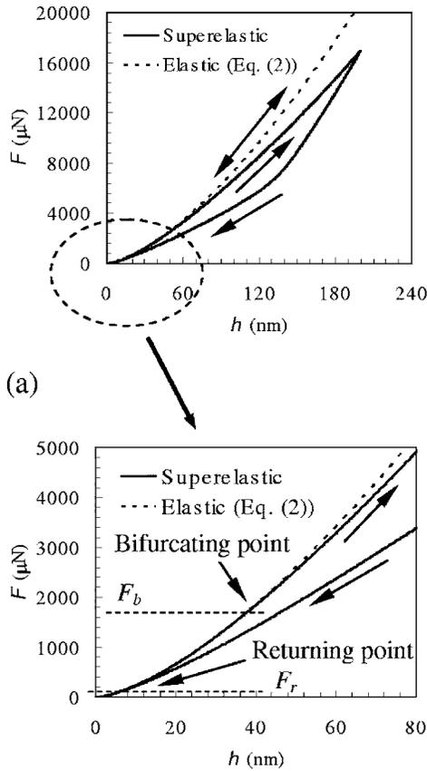
FIG. 2. (a) Comparison between an elastic indentation curve and a superelastic indentation curve, and (b) definitions of the bifurcating point and the corresponding bifurcation force  $F_b$  and the returning point and the corresponding return force  $F_r$ .
