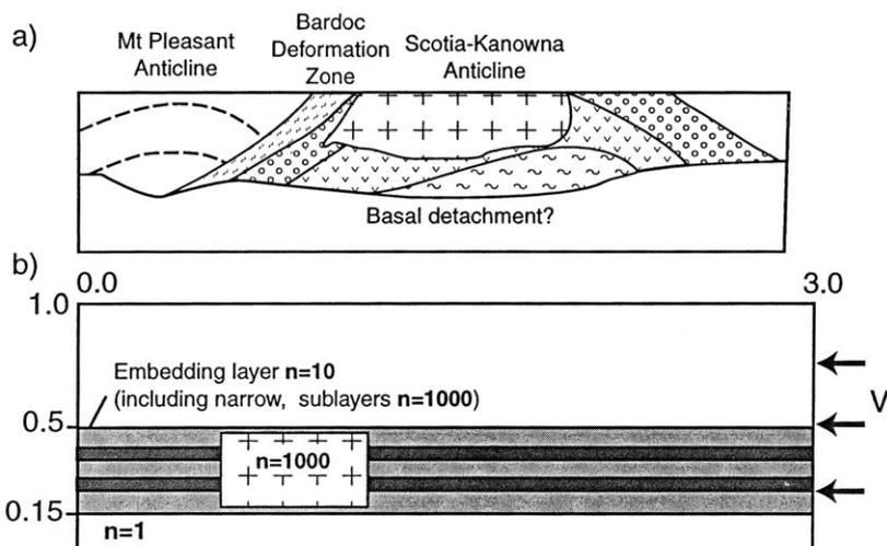
Fig. 3. (a) Seismic interpretation of the shape of a granite pluton and relation to country rocks in the Norseman-Wiluna Belt (after Swager et al., 1997, Fig. 10); (b) initial geometry and set-up of the numerical models. The model box has three wide layers: the bottom layer (viscosity  $n = 1$ ), the middle layer ( $n = 10$  and  $1000$ ), which embeds the rigid granite analogue (high viscosity rectangle,  $n = 1000$ ), and the top layer corresponding to air.
