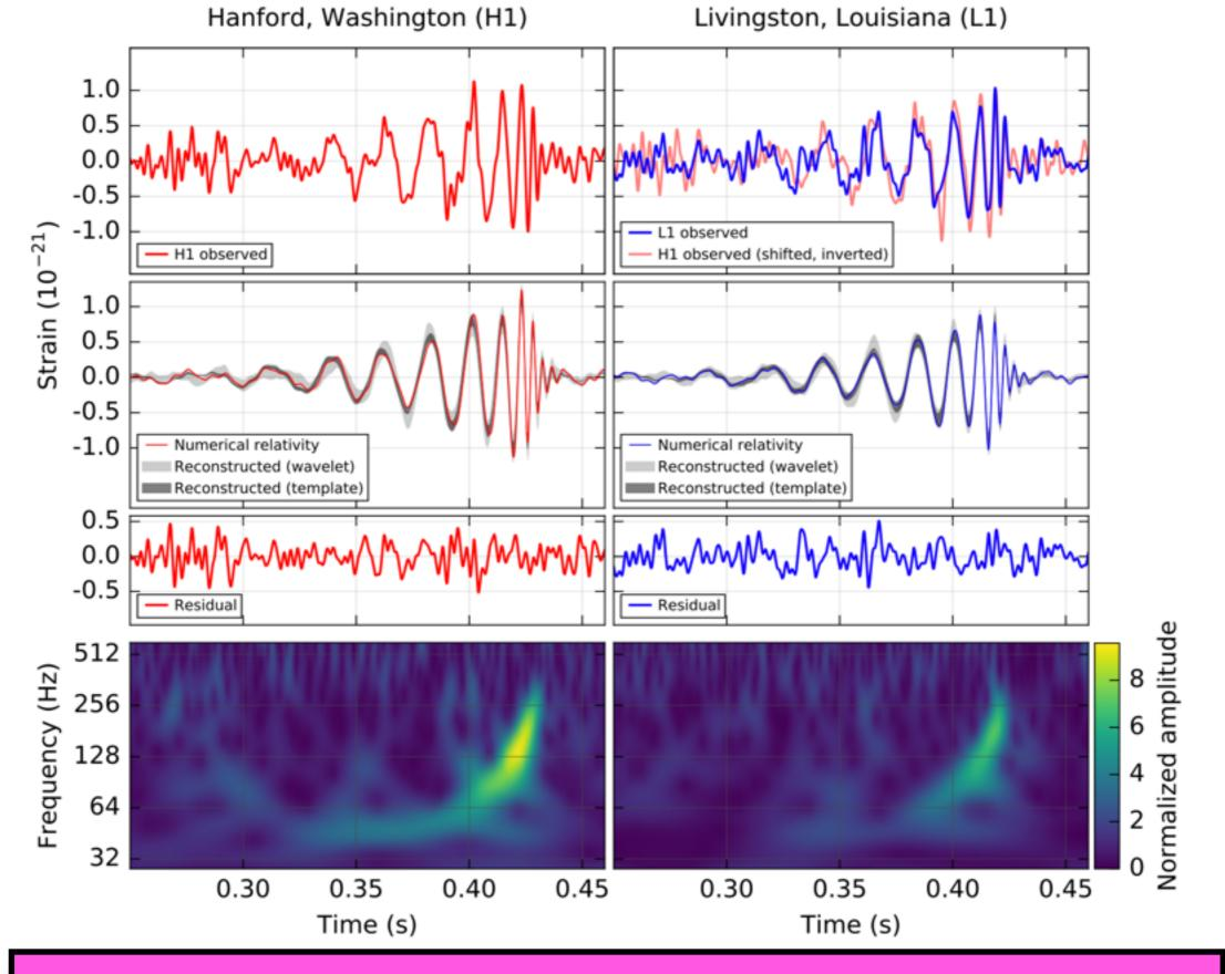
Peak displacement of interferometer arms:  $0.002 \,\mathrm{fm} = 2 \times 10^{-18} \,\mathrm{m}$
