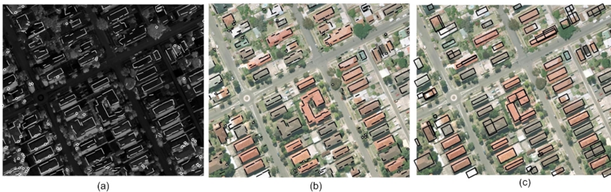
Figure 3: (a) Application of NDVI and (b) line-adjustment to remove tree-edges. Lines with small circles at centres are removed. (c) Initial building positions.
