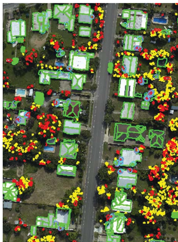
Fig. 13. Results for the AV1 data set. Green: extracted roof planes, other colours: false planes mostly extracted on trees and therefore removed. (For interpretation of the references to colour in this figure legend, the reader is referred to the web version of this article.)
