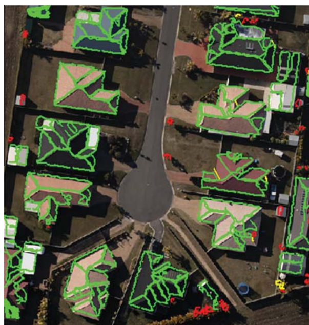
Fig. 14. Results for the HB data set. Green: extracted roof planes, other colours: false planes mostly extracted on trees and therefore removed.
