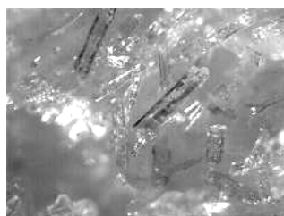
Figure 3: Optical microscope images of salicylic acid needles (left) and 2-ethoxybenzamide (right).
