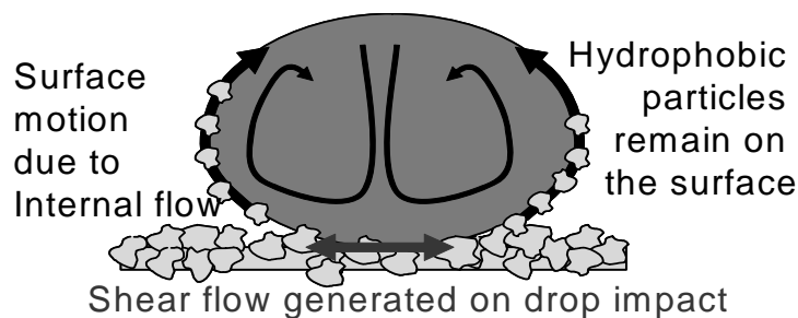
Figure 2: Alternate explanations for the movement of particles around the surface of the drop include surface flow as a result of shear flow at the impact point and/or bulk flow within the drop following impact and deformation.
