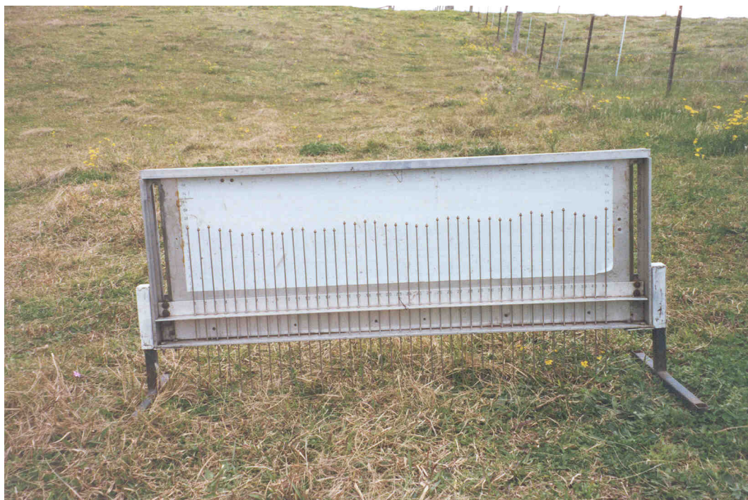
Figure 9.31: Drop pin profiler used for surface roughness measurements.
