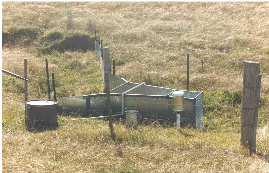
Figure 9.9: Partial flume and raingauges located at the catchment outlet.
