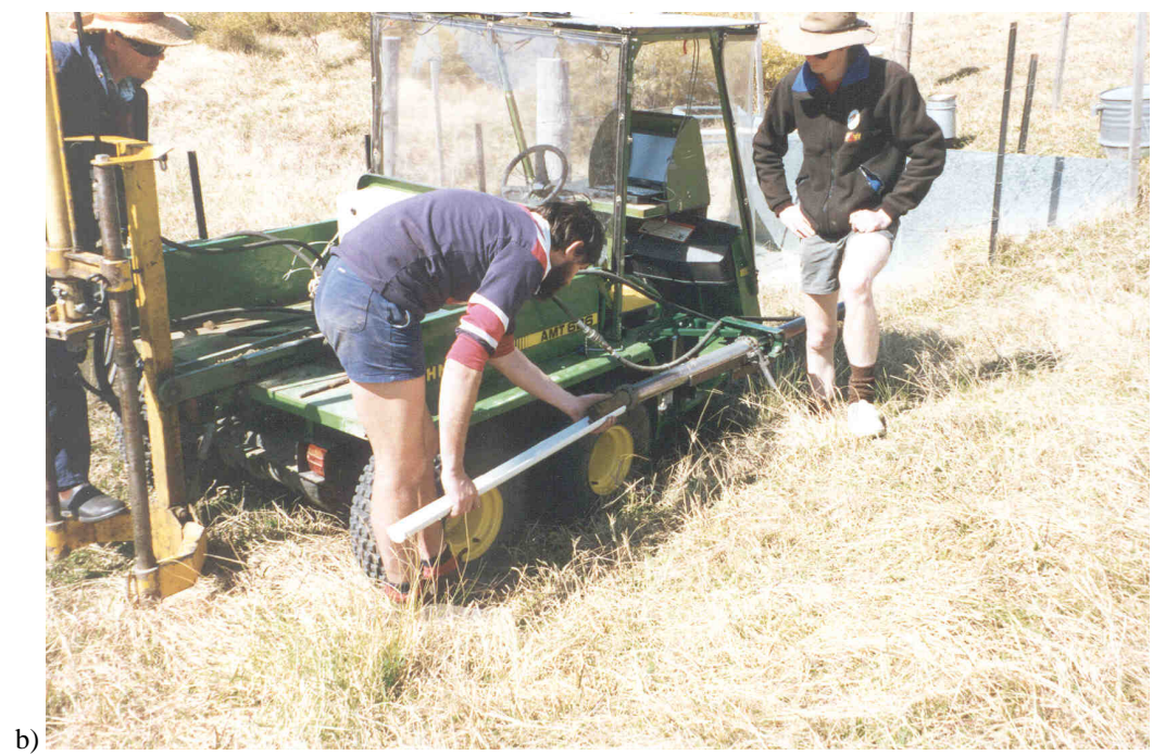
Figure 9.42: The “Green Machine” in a) soil core retrieval and b) soil core extraction modes.
