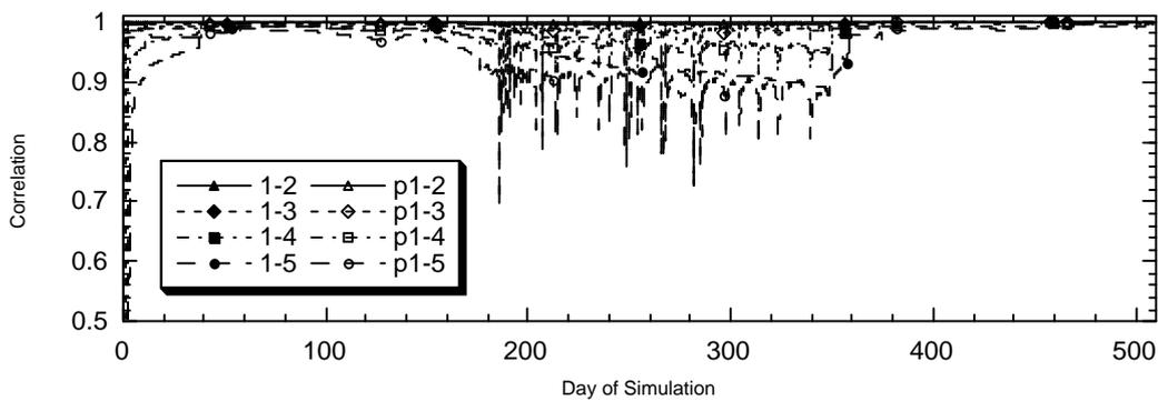
Figure 8.1: Comparison of the predicted (p) correlations (open symbols) using the dynamics simplification approach and the original Kalman-filter estimate of correlations (solid symbols) between the near-surface soil layer (1) and soil layers 2 to 5 for Soil Type 1 (ie. p1-4 is the predicted correlation between soil layers 1 and 4).
