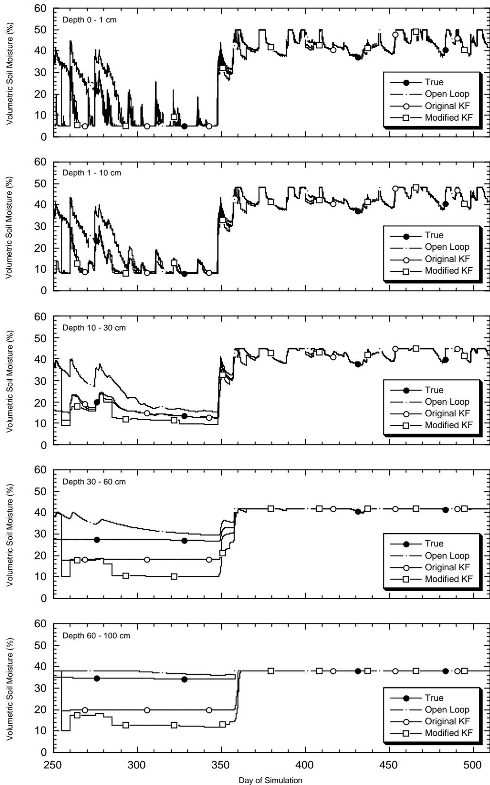
Figure 8.10: Soil moisture profile estimation using the Modified Kalman-filter assimilation scheme with near-surface soil moisture observations over 1 cm depth once every 5 days. Soil Type 2, standard deviations were 5% of the state values.
