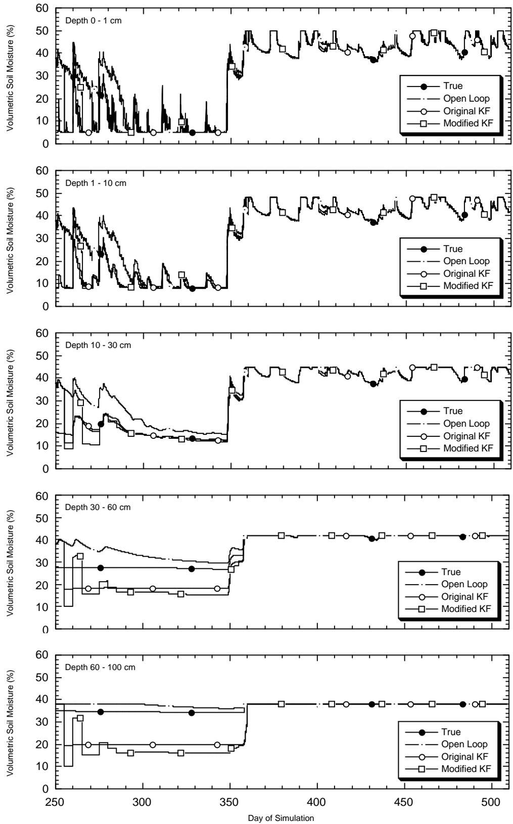
Figure 8.12: Soil moisture profile estimation using the Modified Kalman-filter assimilation scheme with near-surface soil moisture observations over 1 cm depth once every 5 days. Soil Type 2, standard deviations were 5% v/v.
