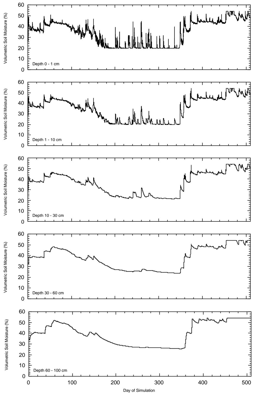
Figure 8.2: Time series of simulated soil moisture content using Soil Type 1 for soil layer depths shown.
