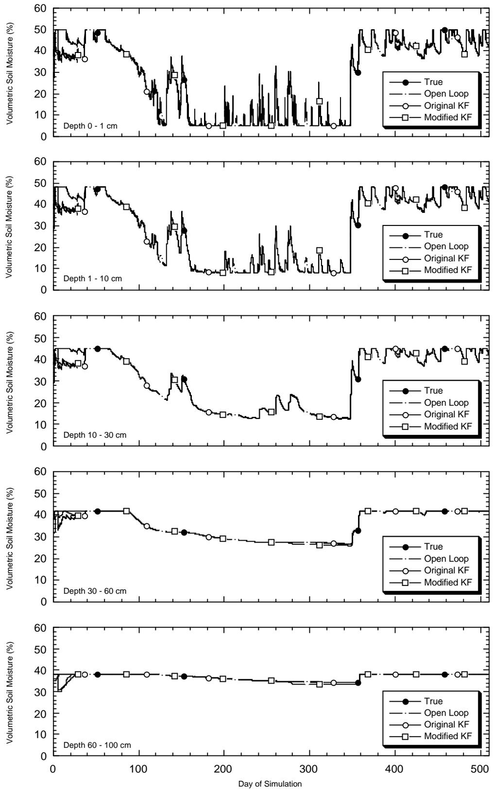
Figure 8.7: Soil moisture profile estimation using the Modified Kalman-filter assimilation scheme with near-surface soil moisture observations over 1 cm depth once every 5 days. Soil Type 2, standard deviations were 5% of the state values.
