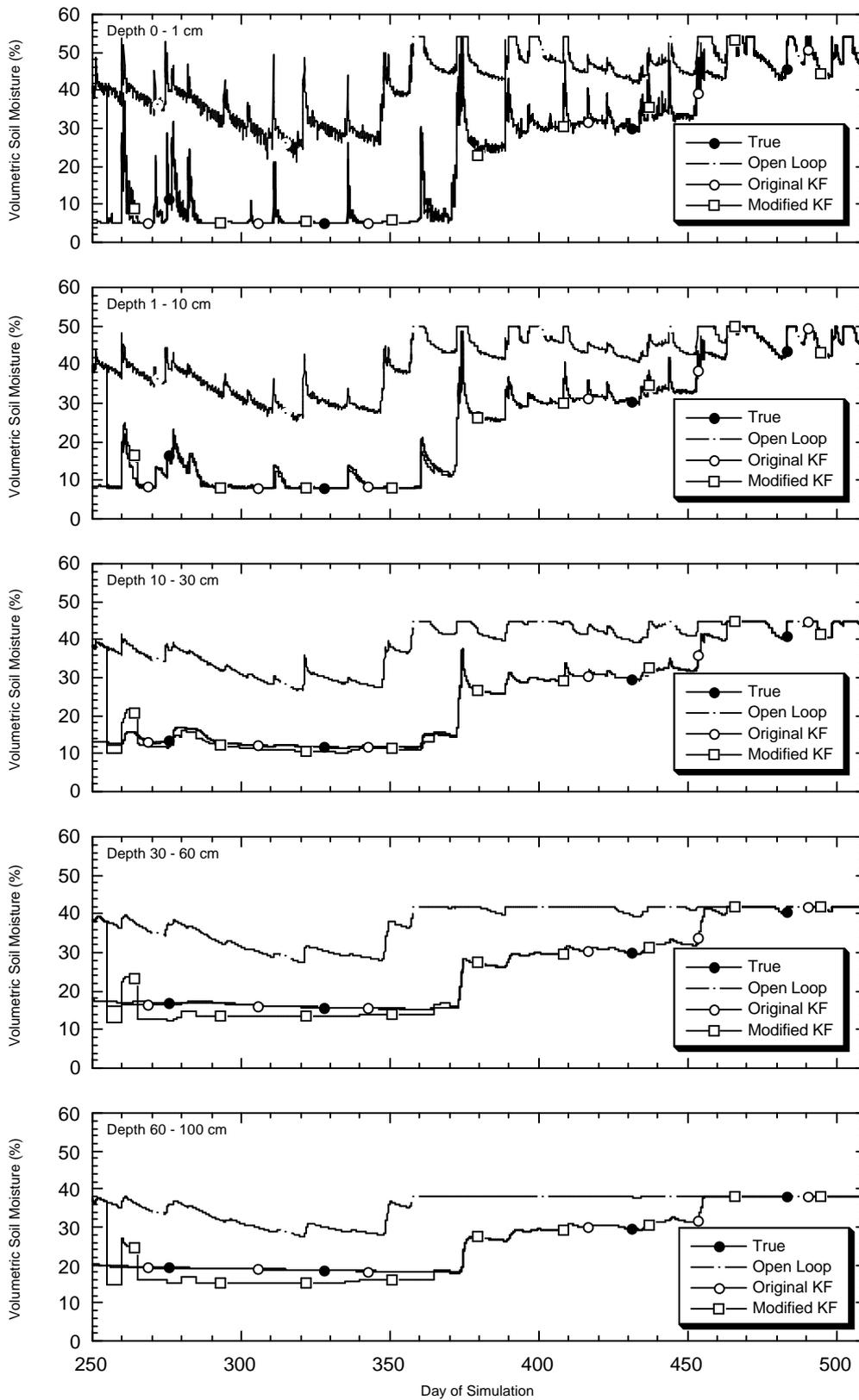
Figure 8.11: Soil moisture profile estimation using the Modified Kalman-filter assimilation scheme with near-surface soil moisture observations over 1 cm depth once every 5 days. Soil Type 3, standard deviations were 5% of state values.
