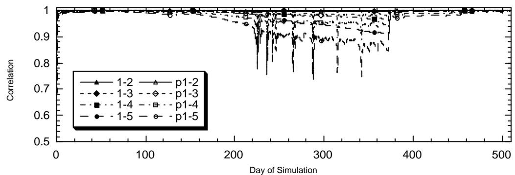
Figure 8.4: Comparison of the predicted (p) correlations (open symbols) using the dynamics simplification approach and the original Kalman-filter estimate of correlations (solid symbols) between the near-surface soil layer (1) and soil layers 2 to 5 for Soil Type 3 (ie. p1-4 is the predicted correlation between soil layers 1 and 4).
