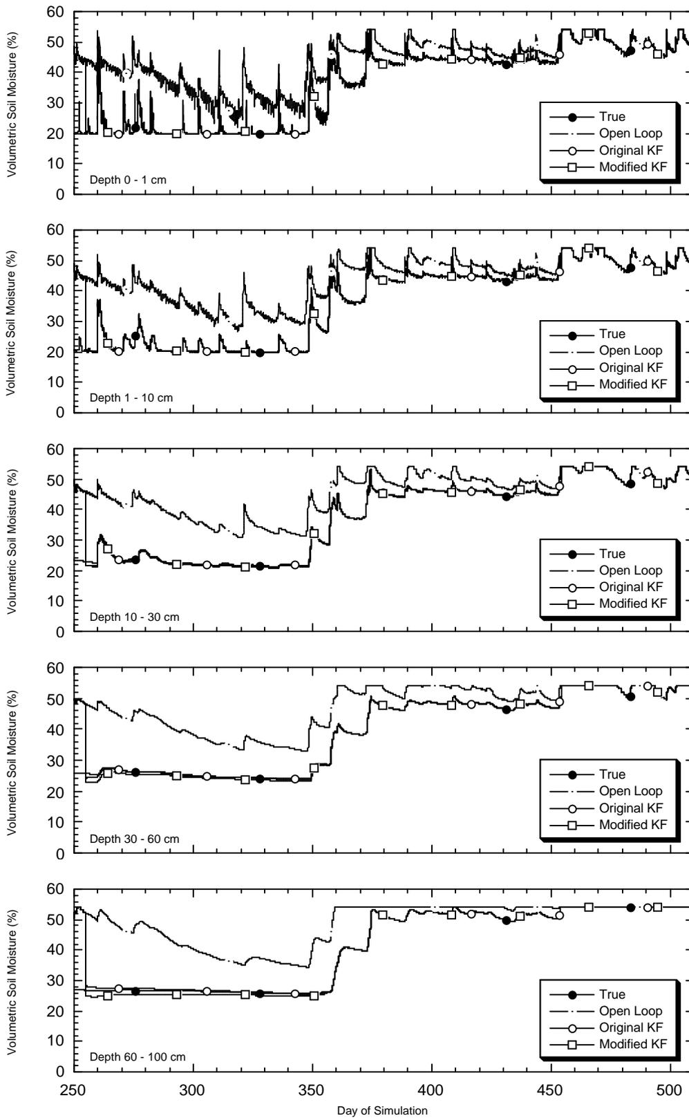
Figure 8.9: Soil moisture profile estimation using the Modified Kalman-filter assimilation scheme with near-surface soil moisture observations over 1 cm depth once every 5 days. Soil Type 1, standard deviations were 5% of the state values.
