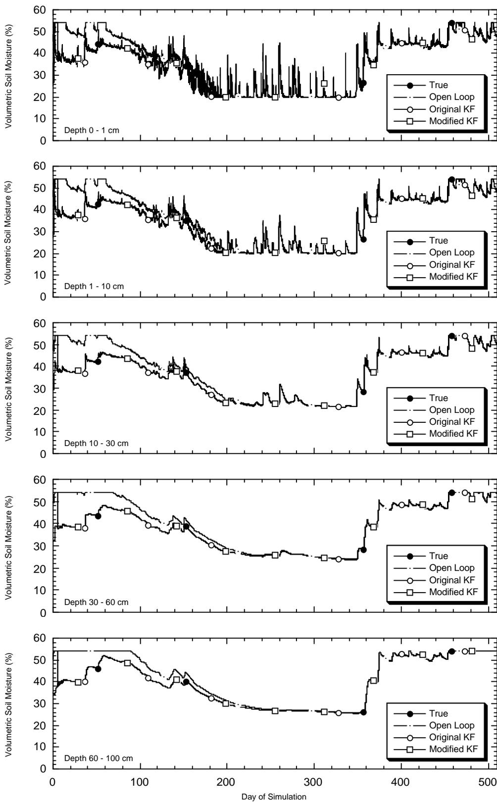
Figure 8.6: Soil moisture profile estimation using the Modified Kalman-filter assimilation scheme with near-surface soil moisture observations over 1 cm depth once every 5 days. Soil Type 1, standard deviations were 5% of the state values.
