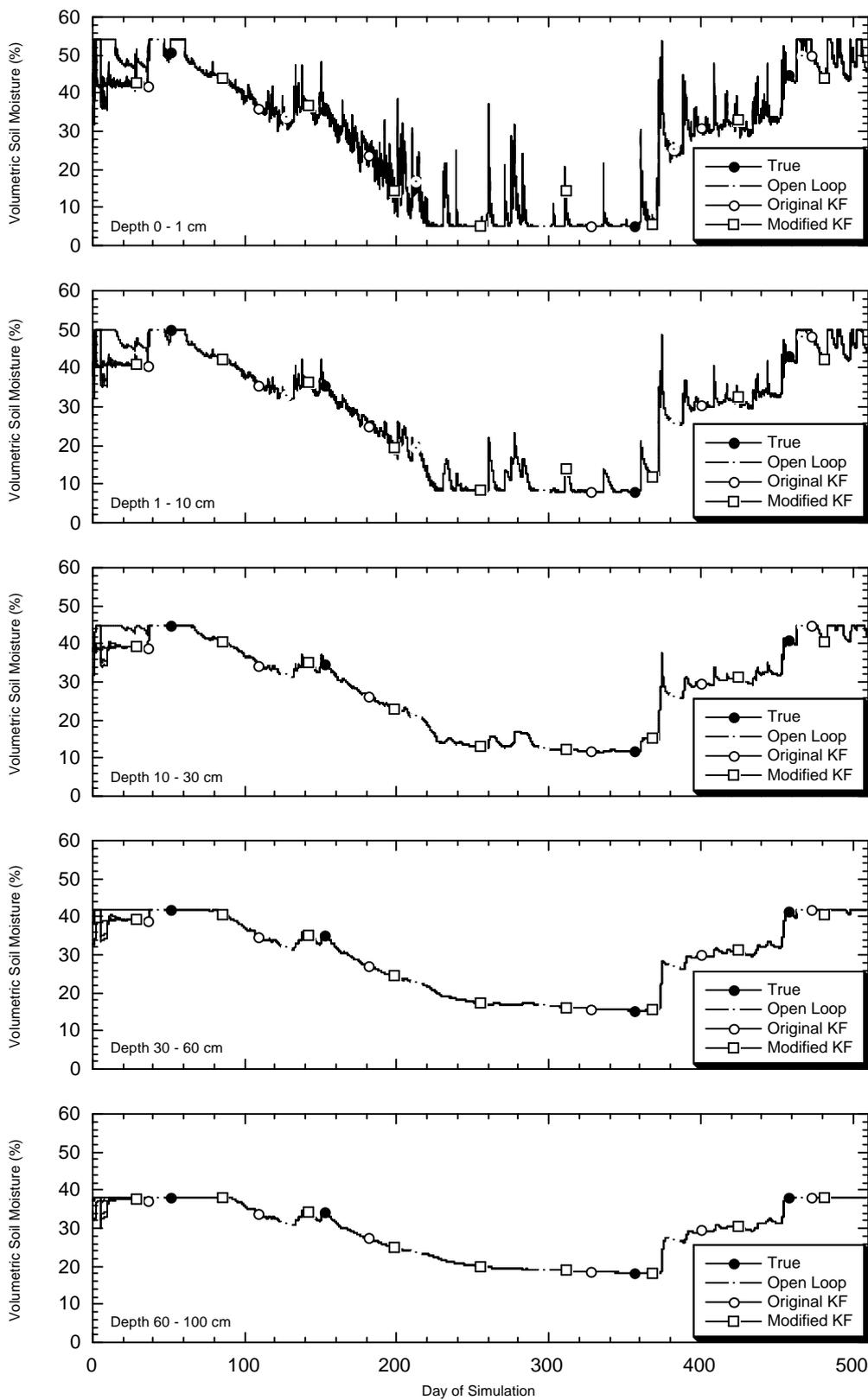
Figure 8.8: Soil moisture profile estimation using the Modified Kalman-filter assimilation scheme with near-surface soil moisture observations over 1 cm depth once every 5 days. Soil Type 3, standard deviations were 5% of the state values.
