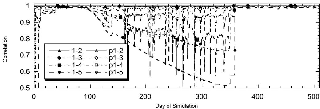
Figure 8.3: Comparison of the predicted (p) correlations (open symbols) using the dynamics simplification approach and the original Kalman-filter estimate of correlations (solid symbols) between the near-surface soil layer (1) and soil layers 2 to 5 for Soil Type 2 (ie. p1-4 is the predicted correlation between soil layers 1 and 4).
