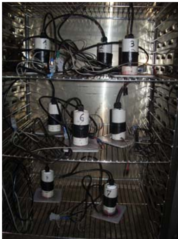
Figure 8 a. drying samples with probes in oven
