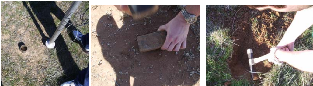
Figure 4.a The ring. b. hammering the ring into ground c. Collecting soil sample for gravimetric analysis
