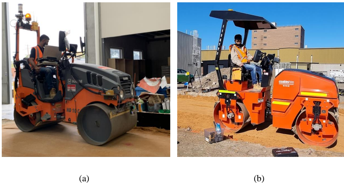
Figure 7-3. Rollers used for this study (a) 1.5t roller for Experiment 1; (b) 4t roller for Experiment 2.
