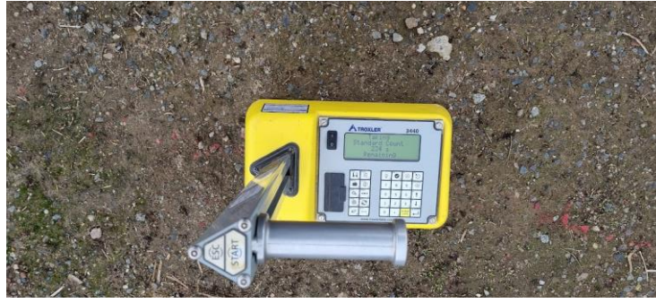
Figure 2-3. Photo of NDG taking the density measurement.
