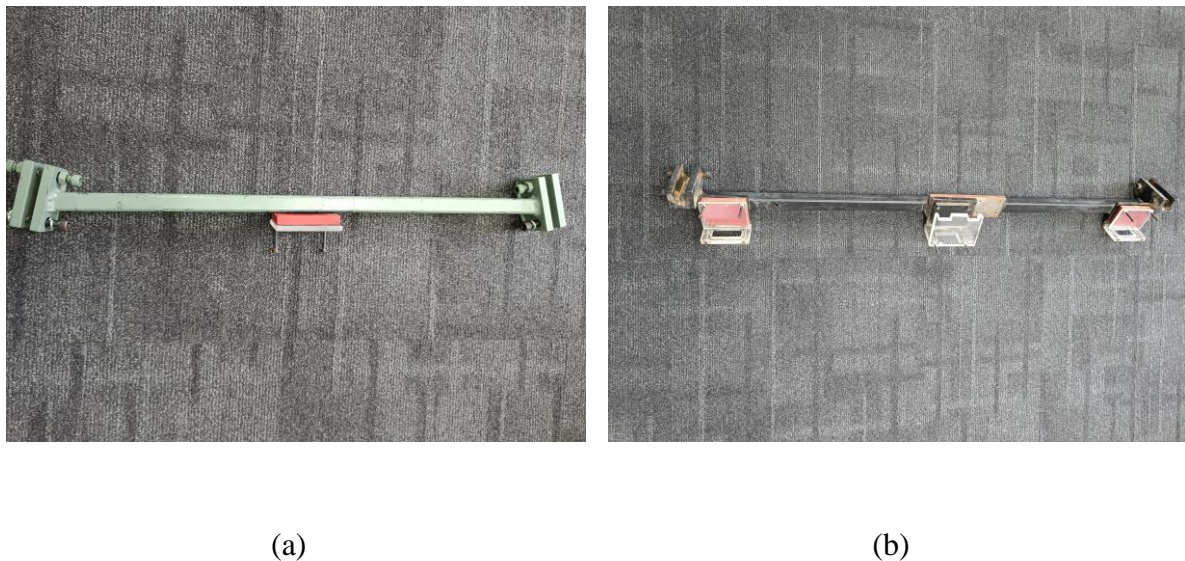
Figure 6-8. Custom designed brackets to install the sensors to the compactor.
