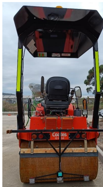
Figure 7-9. Three laser sensors are attached to the back of the roller.
