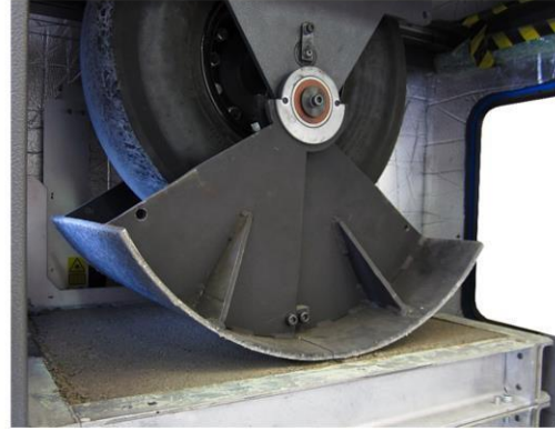
Fig. 4. Photo of the segmented roller and specimen during compaction.
