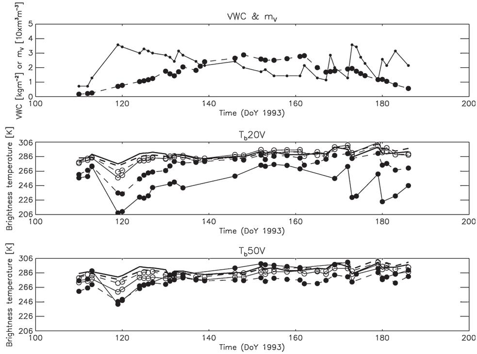
Fig. 2. Example of variables observed over a wheat field during the PORTOS-93 experiment. From top to bottom: VWC and surface soil moisture measured at 2.5 cm ( $m_v$ ) and V-polarized brightness temperatures ( $T_b$ ) at two incidence angles of 20° and 50° for six frequencies (1.41 GHz, closed circles and solid line; 5.05 GHz, closed circles and dashed line; 10.65 GHz, open circles and solid line; 23.8 GHz, open circles and dashed line; 36.5 GHz, solid line; 90 GHz, dashed line).
