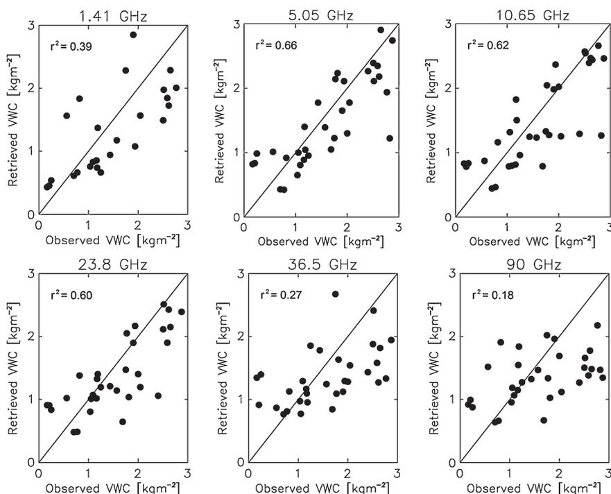
Fig. 3. Retrieved versus observed VWCs at the six frequencies observed, using a biangular approach (50° and 20°) at V polarization, i.e., 50V20V.
