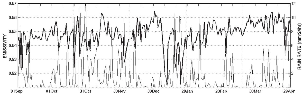
Fig. 5. (Dashed line) Daily mean AMSU-A emissivities at 89 GHz in northern France ( $0.5^{\circ}$  W– $4^{\circ}$  E and  $46^{\circ}$  N– $49^{\circ}$  N) from 01/09/2008 to 30/04/2009 and (solid line) daily precipitation measured *in situ*.
