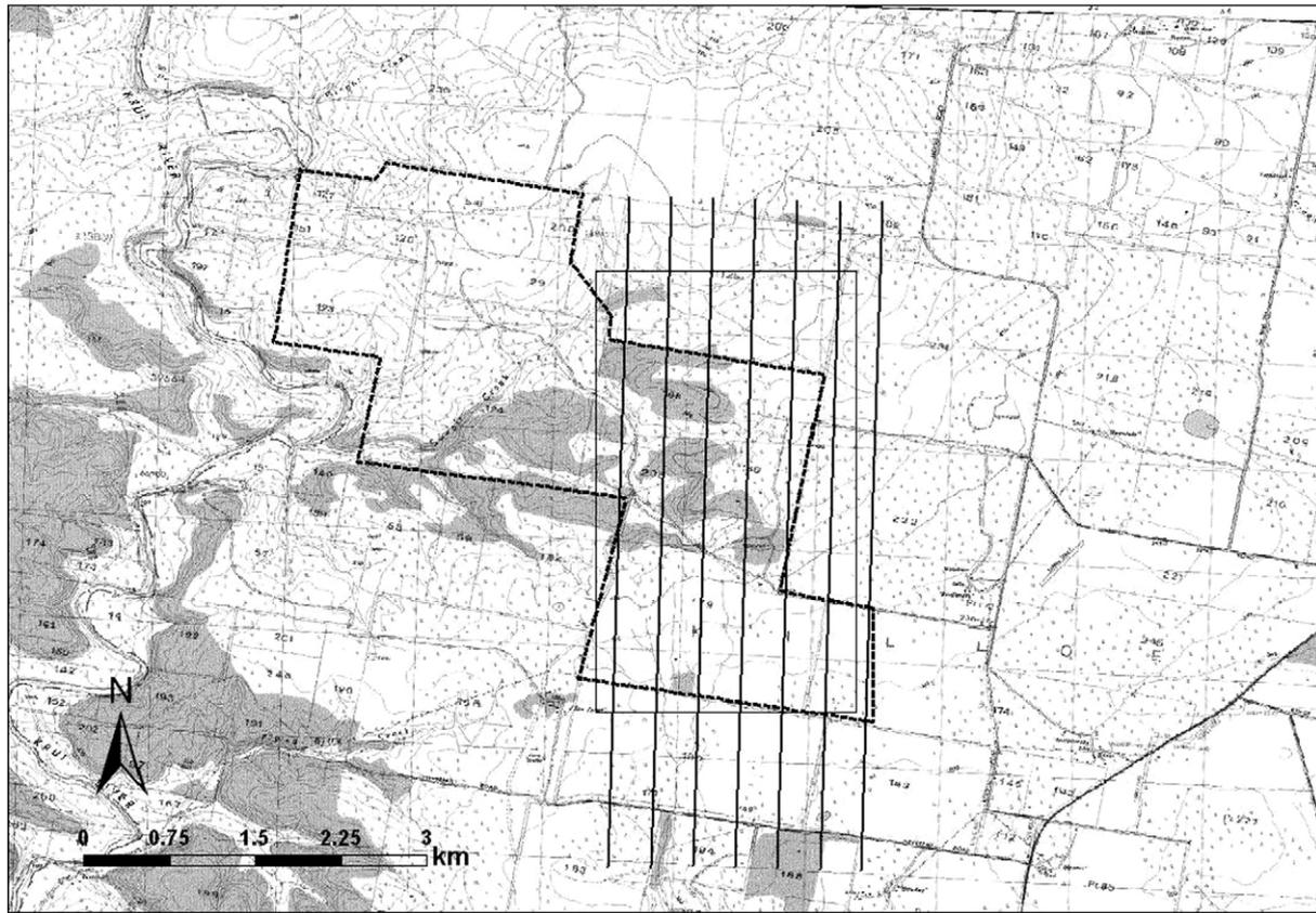
Fig. 1. Topographic map of the area around Roscommon farm. The farm boundary is given by the dotted line, the thick solid lines show the seven PLMR flight lines at approximately 150 m altitude above ground level and the thin-lined rectangle indicates the approximate study area. The forest areas are coloured in grey.
