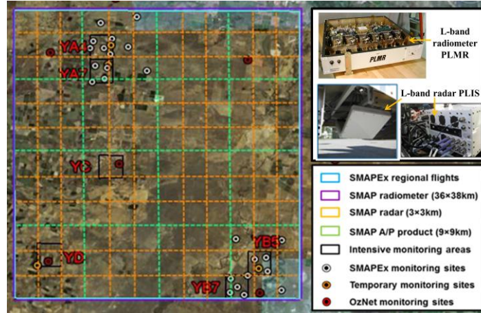
Fig. 1: Overview of the SMAPEX site and its focus areas, with a size of \sim 36\text{km} \times 38\text{km} , approximating one SMAP radiometer pixel. Inset shows the airborne sensors PLMR and PLIS.
