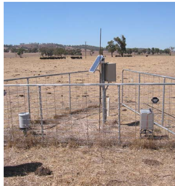
Figure 5. A typical site enclosed by 14 ft gates. Tipping bucket rain gauge in left of enclosure, logger in centre, piezometer slightly to right and gravity meter in far right.
