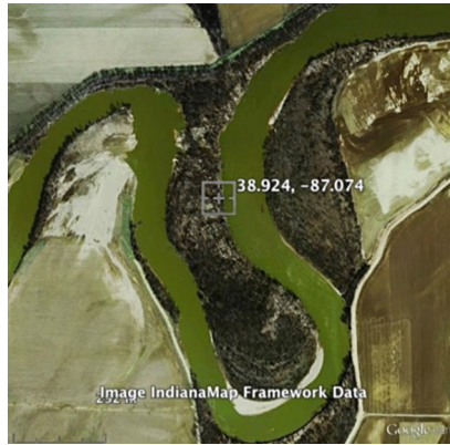
FIGURE 16.4 A meander bend covered by the measurement pixel showing the opportunity for flow area expansion onto the point bars and floodplain as stage and discharge increase.
