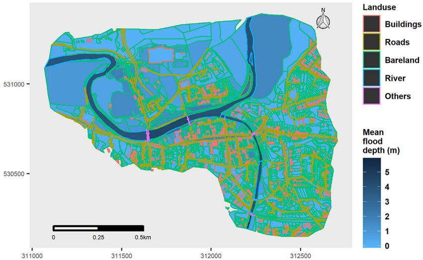
FIGURE 10.1 Land use flood depth map obtained by overlaying predicted 2D flood inundation map and land use map—Storm Desmond floods (5–6/12/2015), Cockermonth, Cumbria, United Kingdom. Attribution statement: Contains OS data © Crown Copyright and database.
