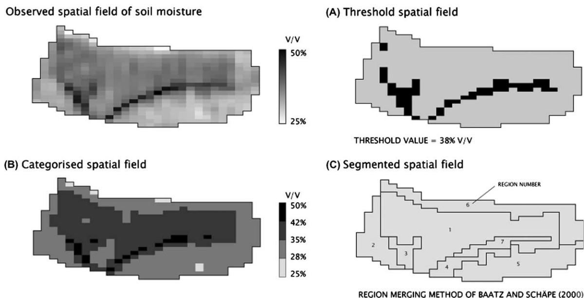
Fig. 1. Identification of regions within a spatial field of soil moisture using three alternate methods: (A) histogram thresholding; (B) histogram slicing; and (C) region merging.
