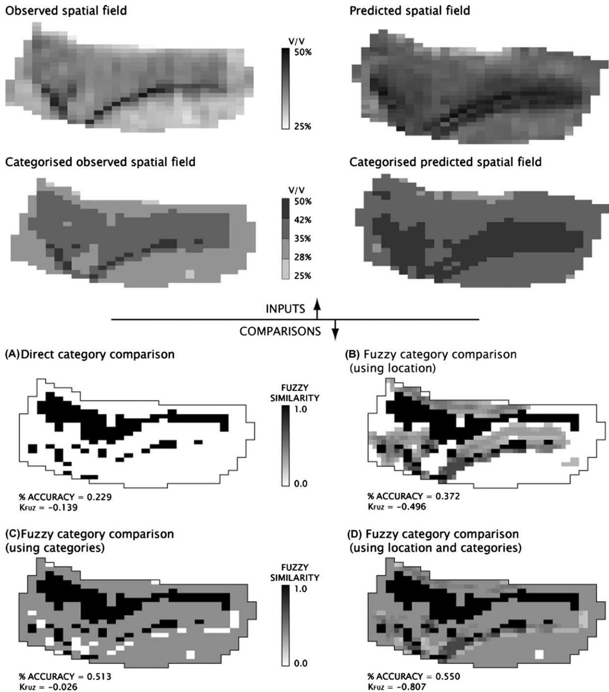
Fig. 3. Fuzzy comparison of observed and predicted spatial fields using four approaches: (A) category comparison; (B) fuzzy comparison with locational tolerance; (C) fuzzy comparison with categorical tolerance; (D) fuzzy comparison with both locational and categorical tolerance.
