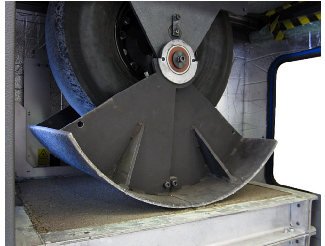
Fig. 4. Photo of the segmented roller and specimen during compaction.
