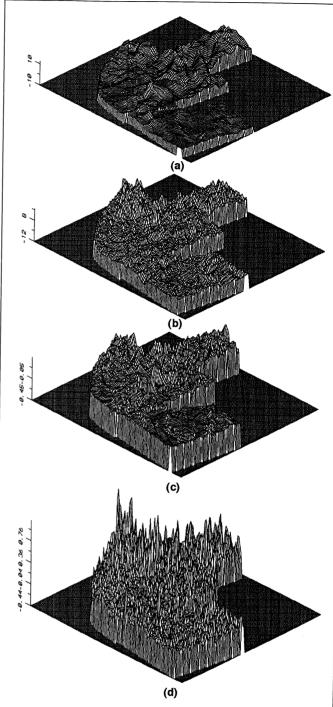
Figure 4. Surface plot of errors in elevation (vertical exaggeration 10): (a) cartometric DEM, (b) photogrammetric DEM: surface plot of errors in slope (vertical exaggeration 500), (c) cartometric DEM, and (d) photogrammetric DEM.
