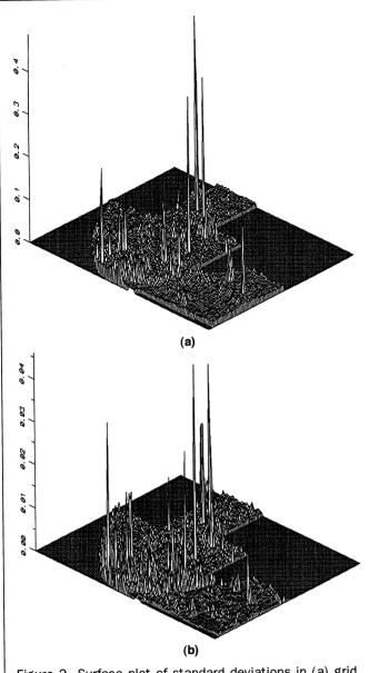
Figure 2. Surface plot of standard deviations in (a) grid elevation (vertical exaggeration 3500) and (b) slope (vertical exaggeration 35000) for the ground truth DEM.
