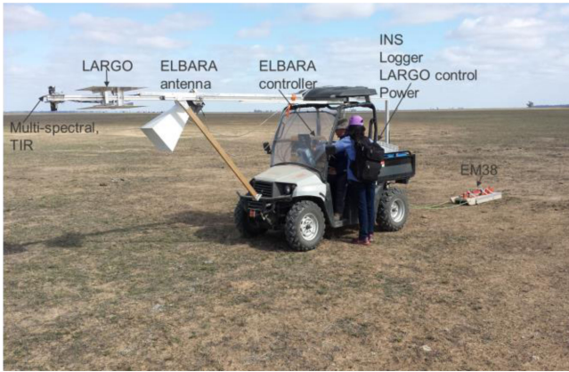
Fig. 1. Buggy platform with multiple sensors, including: an L -band microwave radiometer (ELBARA III), a GNSS-R sensor (LARGO), an electromagnetic induction sensor (EM38), a thermal infrared radiometer, multispectral (VIS/SWIR) sensors and INS, control and power units. Unfortunately technical issues have precluded use of data from the optical instruments in this comparison.
