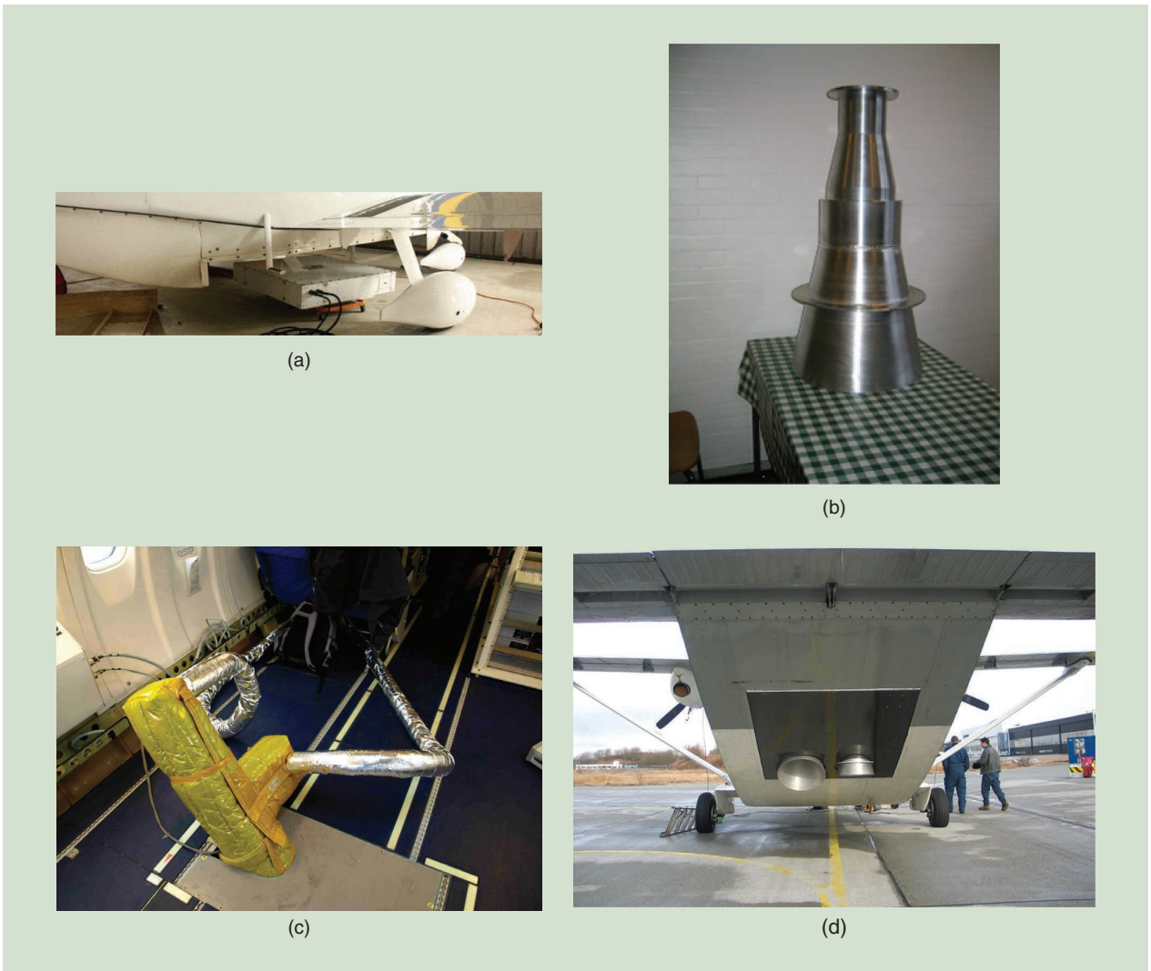
FIGURE 16. (a) A PLMR planar structure. (Source: [104].) (b) A Potter horn antenna used in the CAROLS and EMIRAD radiometers. (Source: [93].) (c) A CAROLS horn antenna installed on an aircraft. (Source: [18].) (d) EMIRAD horn antennas installed on an aircraft. (Source: [93]).
