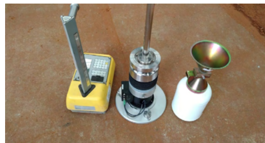
(d) Insitu tests for material density and modulus measurement
