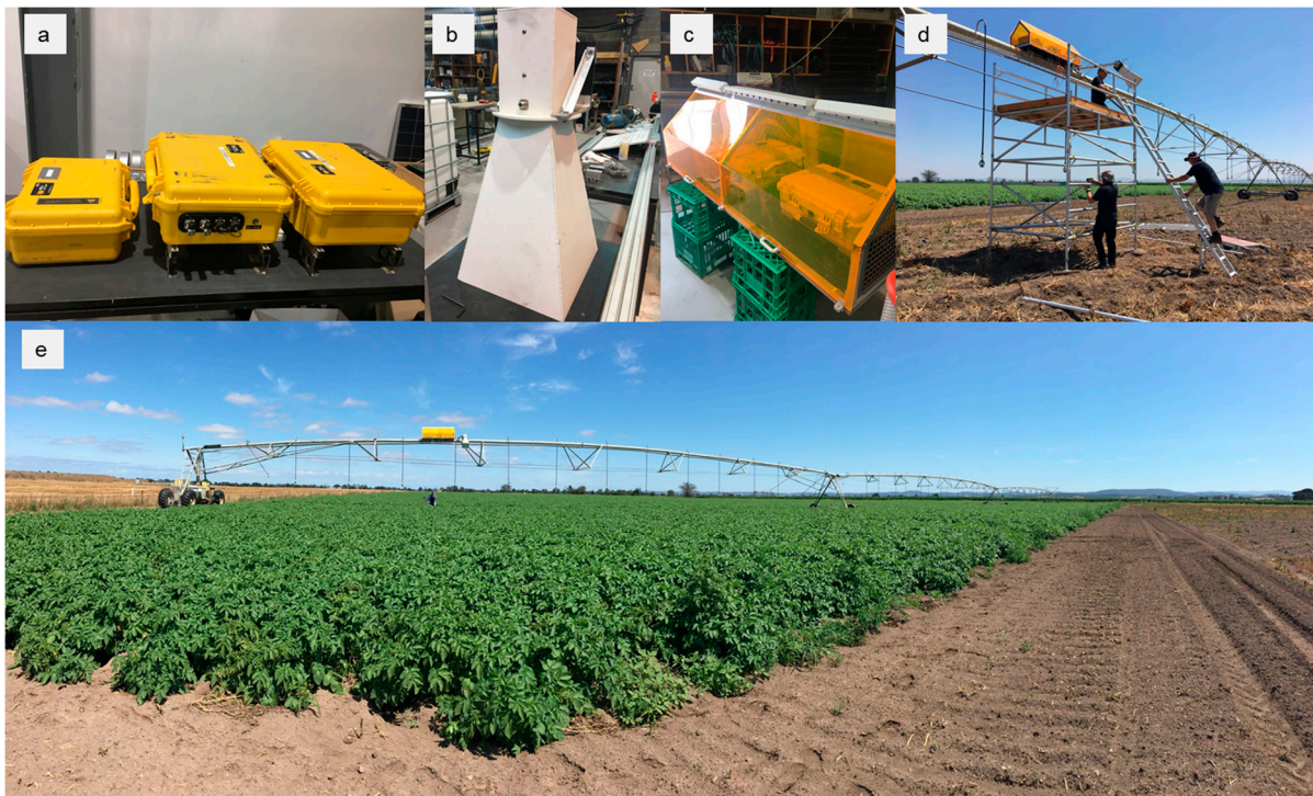
Figure 1. (a) Control unit and battery of the L-band radiometer ELBARA; (b) Horn antenna of ELBARA; (c) Waterproof house of ELBARA components; (d) Setup of ELBARA system onto a linear shift irrigator; and (e) Soil moisture monitoring over a potato farm by the Smart Irrigation System.
