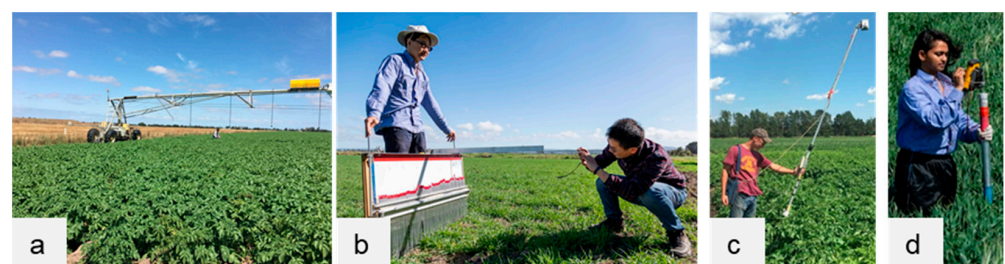
Figure 3. Instruments used during the farm experiment, including (a) ELBARA radiometer mounted on a linear shift irrigator, (b) a roughness pin profiler, (c) a spectral radiometer for vegetation index, and (d) HDAS for soil moisture monitoring as ground truth.
