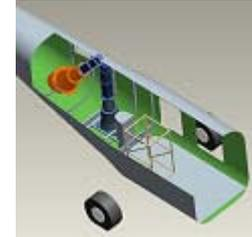
Layout design of the antenna horn
