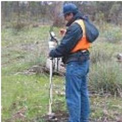
Taking ground measurements of near-surface soil moisture
