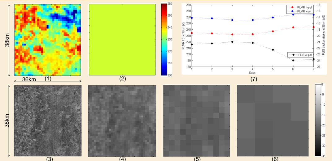
**Fig. 3:** An example of PLMR (h-pol) and PLIS (vv-pol) data observed concurrently from SMAPEX-3: (1) PLMR TB observed at 1km; (2) PLMR upsampled to 36km; (3) PLIS  $\sigma^{\circ}$  observed at 10m, and then upsampled to (4) 1km, (5) 3km and (6) 9km; (7) time-series of PLMR and PLIS data at 36km across 7 days.
