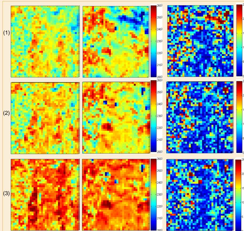
**Fig. 6:** Comparison between (a) downsampled TB and (b) PLMR observations at h-pol and 1km resolution; The difference of each 1km pixel results for 3 days: Day2 (1), Day5 (2) & Day9 (3) is shown in (c).
