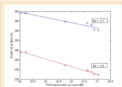
**Fig. 5:**  $\beta$  estimation from linear regression:  $\beta = -3.9$  from TB at h-pol and  $\sigma^{\circ}$  at vv-pol;  $\beta = -2.7$  from TB at v-pol and  $\sigma^{\circ}$  at vv-pol.
