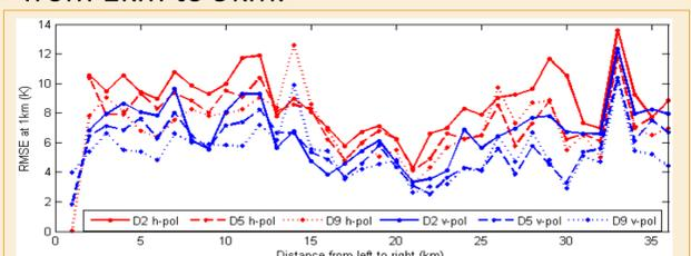
**Fig. 7:** RMSE of each 1km strip of Day2, Day5 & Day9 vs the distance starting from left to right: red lines are RMSE of downsampled results at h-pol, while the blue lines are RMSE of downsampled results at v-pol.
