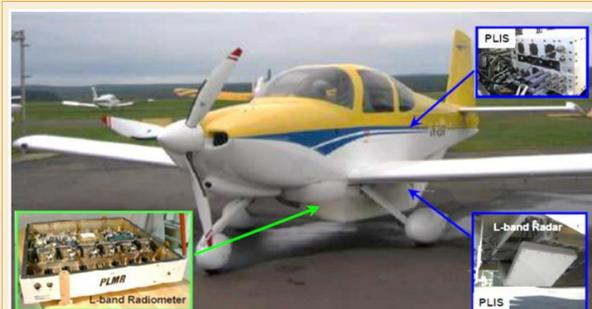
**Fig. 2:** Airborne simulator including Polarimetric L-band Multibeam Radiometer (PLMR); and the Polarimetric L-band Imaging Synthetic aperture radar (PLIS).
