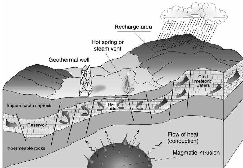
Figure 2: Schematic of a typical geothermal project (Barbier, 2002)
