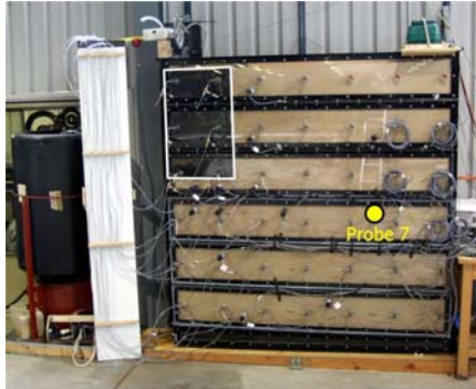
Figure 2: 2D laboratory infiltration system
