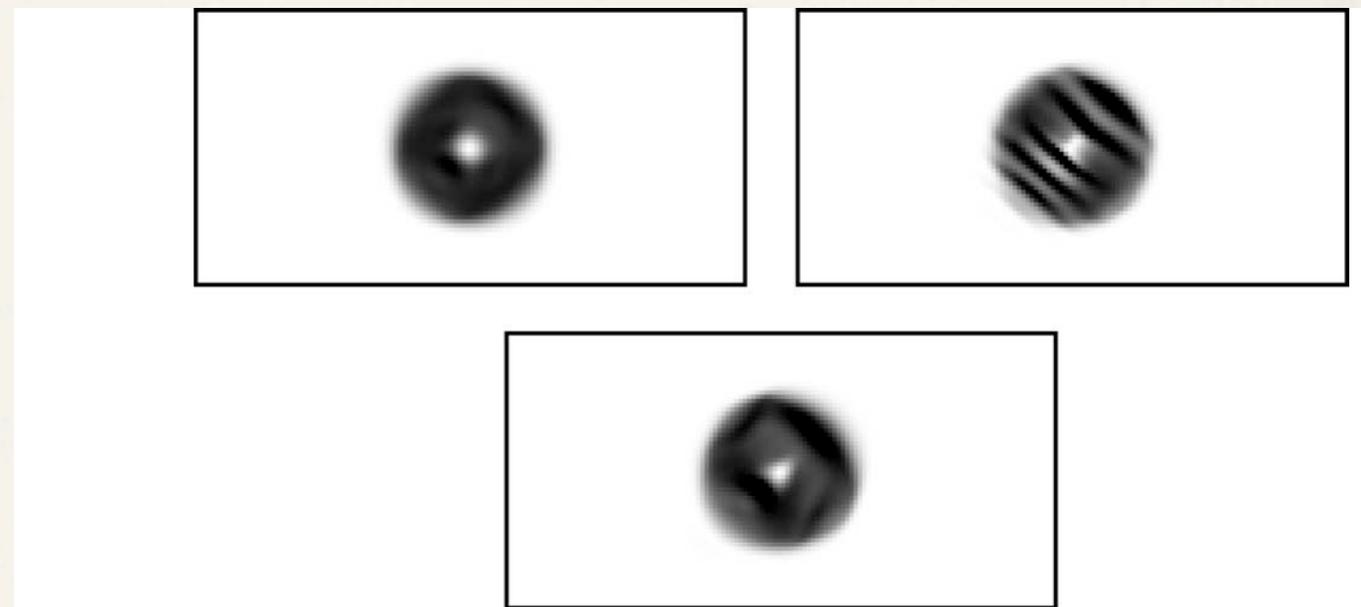
Fig. 3. Gray-scale images of the magnetic pressure  $(B_x^2 + B_y^2)$  at  $t = 2$  for an advected field loop ( $v_0 = \sqrt{5}$ ) using the  $\mathcal{E}_z^a$  (top left),  $\mathcal{E}_z^c$  (top right) and  $\mathcal{E}_z^c$  (bottom) CT algorithm.
