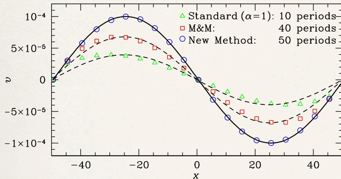
**Figure 2.** As Fig. 1, but for SPH with standard ( $\alpha = 1$ ) or Morris & Monaghan (1997) artificial viscosity, as well as our new method (only every fifth particle is plotted). Also shown are the undamped wave (*solid*) and lower-amplitude sinusoidals (*dashed*). Only with our method the wave propagates undamped, very much like SPH without any viscosity, as in Fig. 1.
