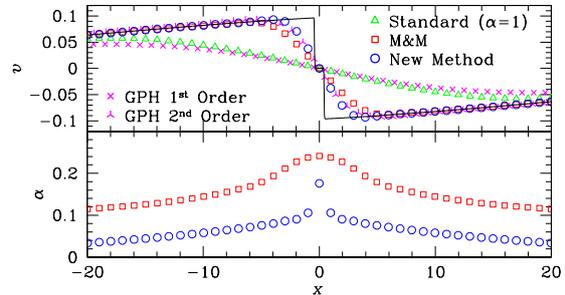
**Figure 6.** Steepening of a 1D sound wave: velocity and viscosity parameter vs. position for standard SPH, the M&M method, our new scheme, and Godunov particle hydrodynamics of first and second order (GPH, Cha & Whitworth 2003), each using 100 particles per wavelength. The solid curve in the top panel is the solution obtained with a high-resolution grid code.
