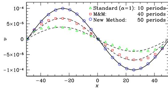
**Figure 2.** As Fig. 1, but for SPH with standard ( $\alpha = 1$ ) or Morris & Monaghan (1997) artificial viscosity, as well as our new method (only every fifth particle is plotted). Also shown are the undamped wave (*solid*) and lower-amplitude sinusoids (*dashed*). Only with our method the wave propagates undamped, very much like SPH without any viscosity, as in Fig. 1.
