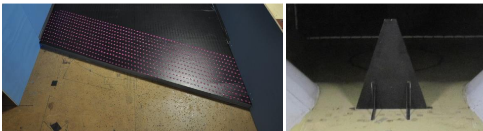
Figure 3. (Left) Surface shear stress visualisation setup. Flow is from bottom to top. Step height is 50 mm. End plates are used. (Right) Trapezoidal vortex generator used to increase boundary layer thickness and turbulence intensity.
