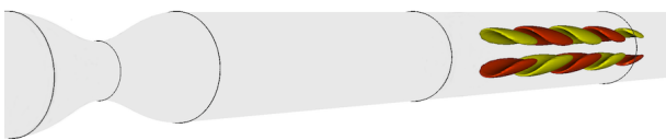
Figure 8: Positive/negative isosurfaces of axial velocity perturbation to steady stenotic flow at time of maximum gain, t = \tau = 6.71 resulting from the inflow boundary perturbation shape shown in figure 7.
