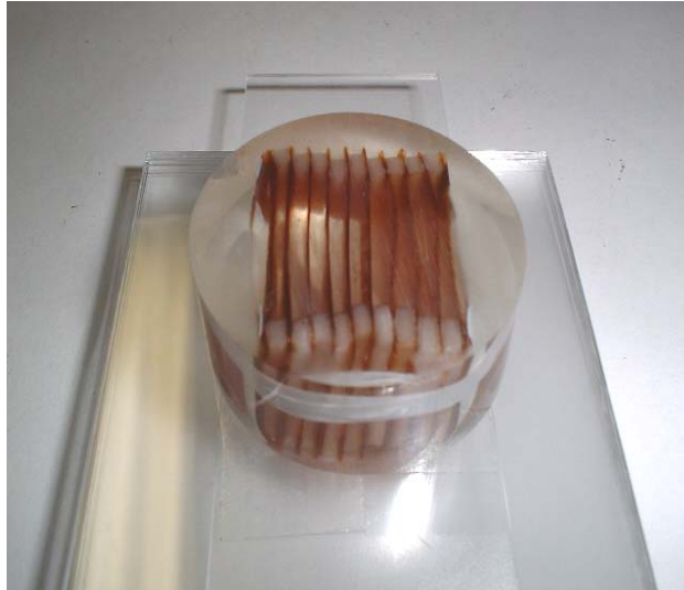
Figure 4-2 Embedded sample ready for examination in confocal microscope
