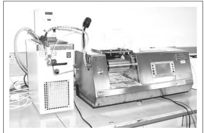
**Fig. 1** Photograph of Hydroscope instrument, showing the two brass rollers, the upper black rubber roller placed in contact with the back brass roller and white tubing through which fountain solution is applied dropwise onto the front roller before entering the nip. The unit on the left controls the temperature of the brass rollers.
