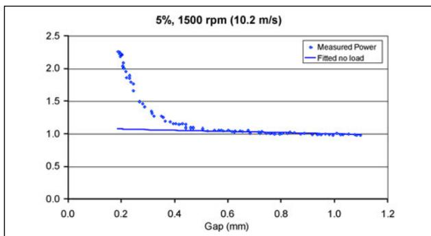
**2. Refiner net power as function of bar clearance at 5% consistency for 1500 rpm and for pulp that had been refined to 283 kW-h/ton. The solid line indicates the linear trend fitted to the no-load power.**
