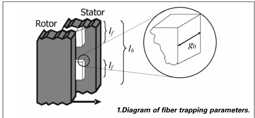
1. Diagram of fiber trapping parameters.
