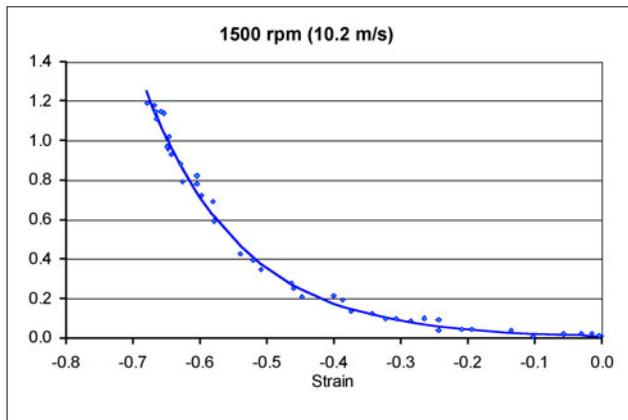
**4. Net refining power as a function of compressive strain level for refining a 5% consistency suspension of the ECF pulp at 1500 rpm.**
