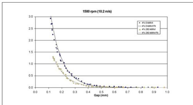
**5. Refiner loading measurements made at 4% consistency and 1500 rpm using unrefined pulp and pulp refined to 283 kW-h/ton.**
