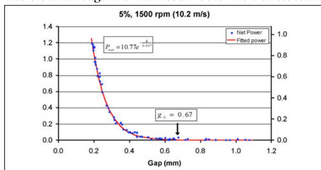
**3. Net refining power vs. gap for a 5% consistency suspension of ECF pulp running the long medium fillings at 1500 rpm.**
