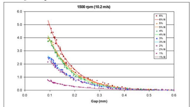
**6. Refiner loadability trials of unrefined pulp for refining at 1500 rpm and consistencies ranging from 1-6%.**
