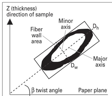
1. Definition of the fiber shape factor and twist angle.
