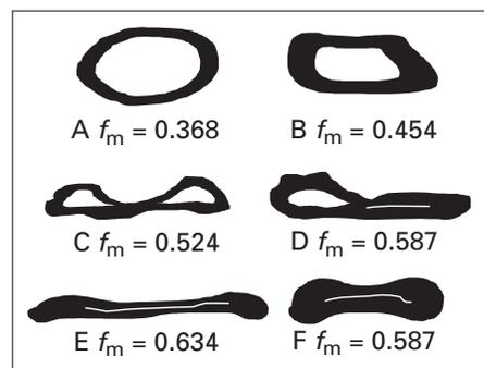
3. Different collapse states of fiber: uncollapsed fibers (A, B), partially collapsed fibers (C, D), and fully collapsed fibers (E, F).
