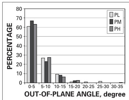
8. The frequency distribution of out-of-plane angle of Samples  $P_L$ ,  $P_M$ , and  $P_H$
