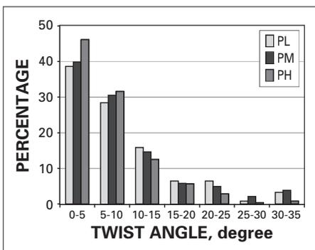
5. Frequency distribution of twist angle of fiber cross section.
