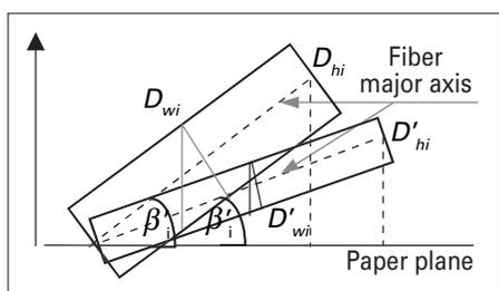
4. In any layer of a sheet, fiber twist and fiber collapse contribute to the reduction in paper thickness.
