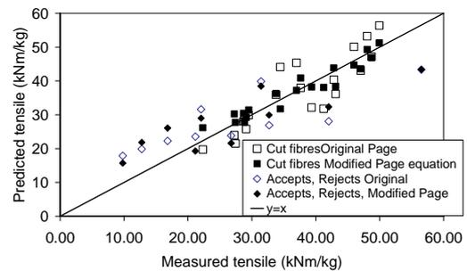
**Figure 4 Tensile strength predicted from the modified (equation 8 and original (equation 5) Page equations vs. measured tensile strength for the cut fibres (L0-L3) series and the Accepts and Rejects from the APPI data**
