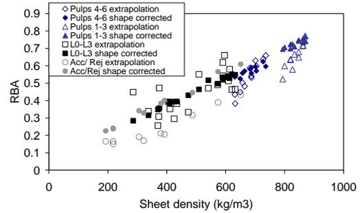
**Figure 3 Comparison of RBA either by the Ingmanson-Thode extrapolation method (hollow points) or by the shape correction method for density (equation 6 with  $(I-r) = 3/4$ ) (solid points)**
