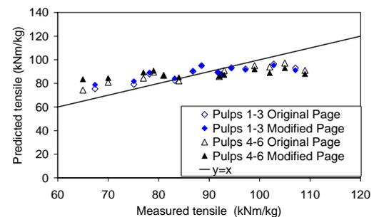
**Figure 5 Tensile strength predicted from the modified (equation 8) and original (equation 5) Page equations vs. measured tensile strength for the pulps 1-6 for the ensis-Papro data**
