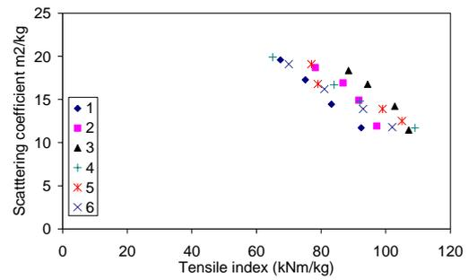
**Figure 1 Scattering coefficient versus tensile strength for the Ensis-Papros data.**
