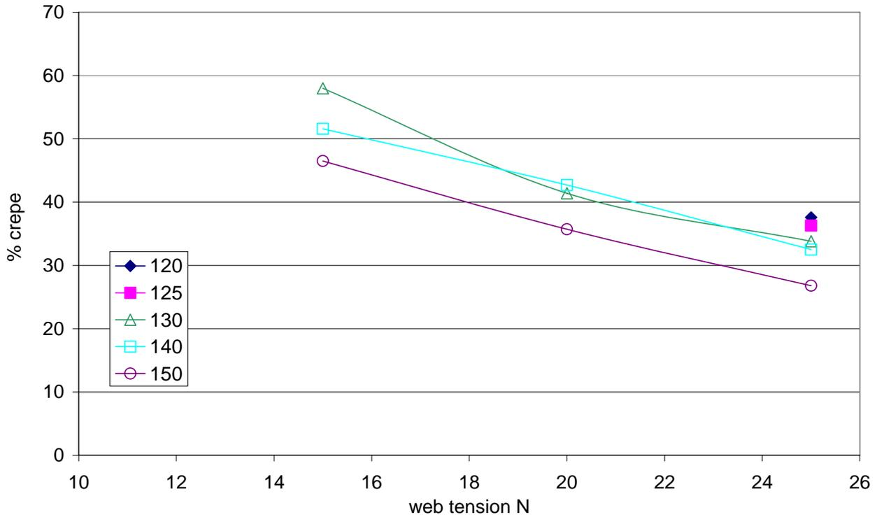
**Figure 2 crepe % as a function of web tension at different temperatures for a 300 mg/m<sup>2</sup> adhesive addition rate to the surface**
