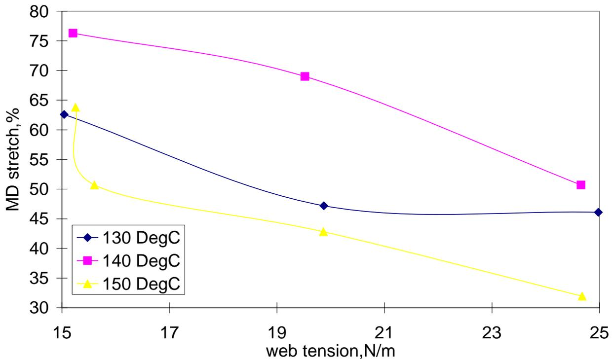
**Figure 5** MD stretch at break (%) as a function web tension and cylinder temperature for an adhesive addition rate of 300 mg/m<sup>2</sup>.
