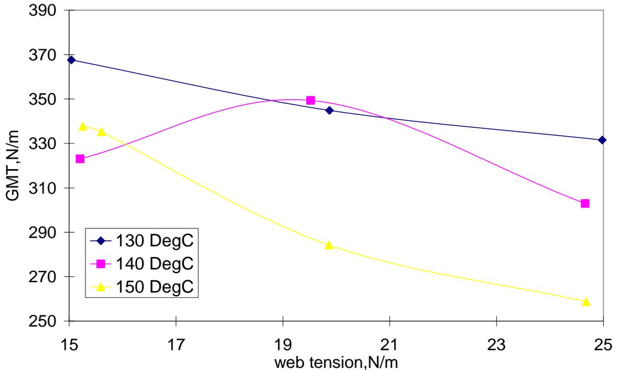
**Figure 3 Geometric Mean Tensile strength (GMT) as a function of web tension and cylinder temperature for an addition rate of 300 Mg/m<sup>2</sup>.**
