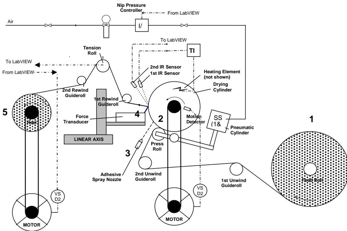
**Figure 1. Pilot-scale creping rig schematic layout.**
