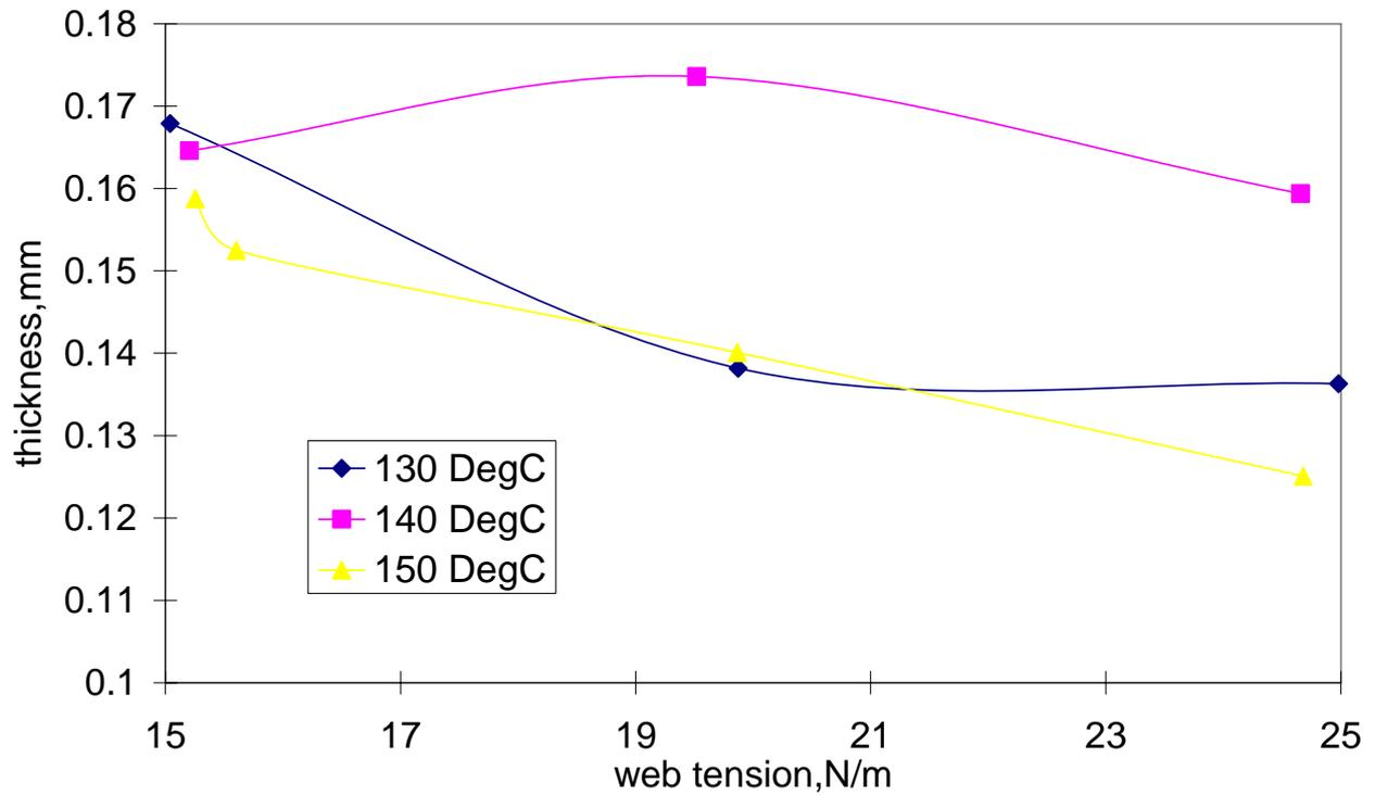
**Figure 4** Sample thickness as a function web tension and cylinder temperature for an adhesive addition rate of 300 mg/m<sup>2</sup>.
