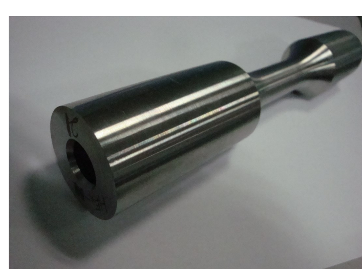
Specimen type 2: Thin-walled tubular specimens ((ASTM E2207-02)
