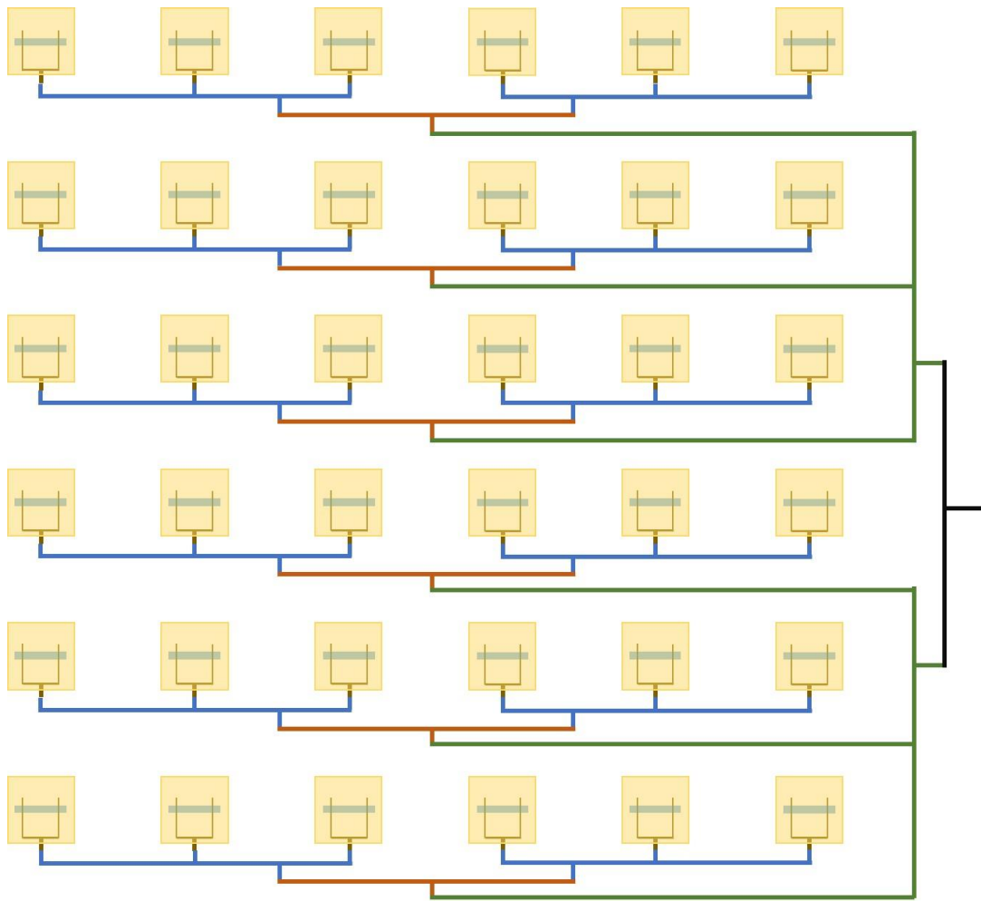
Figure 5. 10 6x6 Feed network case 3 using three-way power dividers at the antenna feed end
