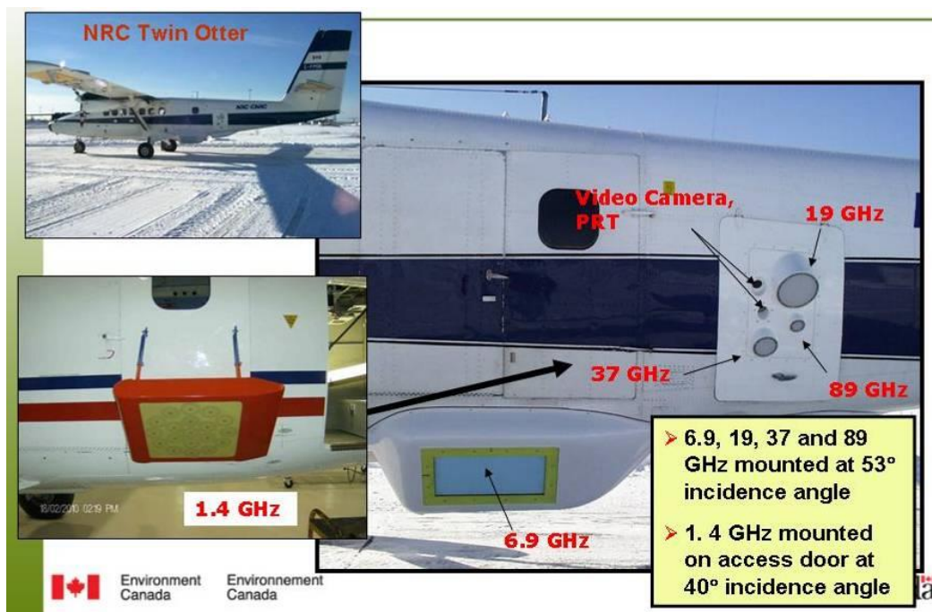
Figure 2. 4 Installation of EC Radiometer on Twin Otter airplane [99]
