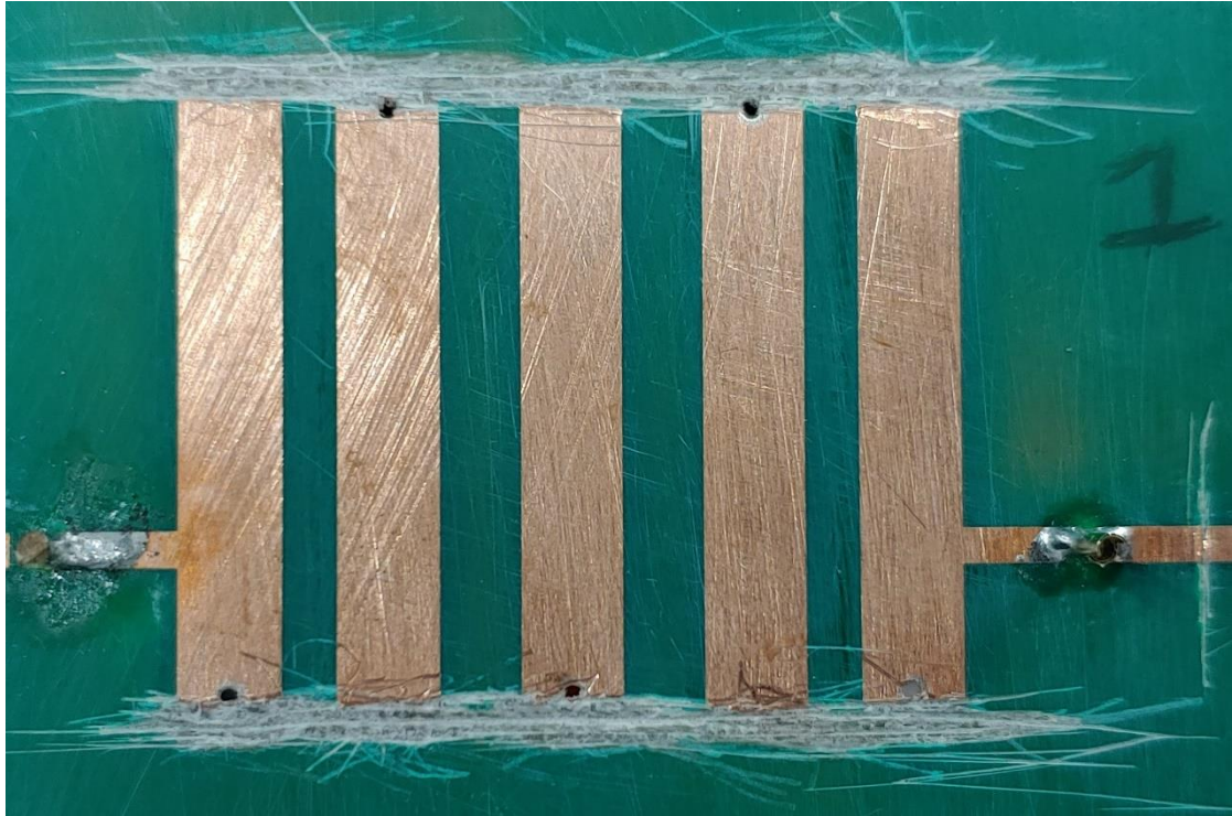
Figure B. 35 The single bandpass filter with final cutting
