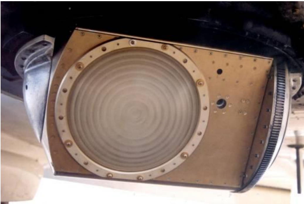
Figure 2. 3 Scanning head installation of PSR/CX [94]
