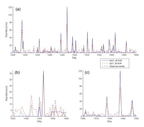
FIGURE 3.8: Panel (a) shows a time series comparison of the reconstructed DCT and DWT signals for the Leaf River (Collins) catchment using 20 POP for a period of 200 days. Panels (b and(c) are smaller windows of the same time series during both low- and high-rainfall periods.
