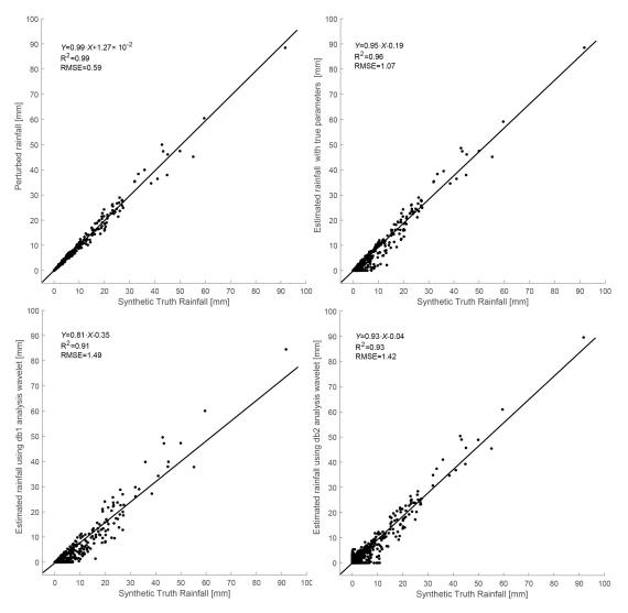
FIGURE 4.2: Comparison of the (top left) perturbed synthetic truth rainfall, and (top right) synthetic and estimated rainfall using inference of only the wavelet parameters (top right plot), joint inference of the SAC-SMA model parameters and wavelet parameters using (bottom left) the db1 wavelet and (bottom right) db2 wavelet. The linear least squares fit and corresponding quality of fit metrics are separately indicated in each plot.
