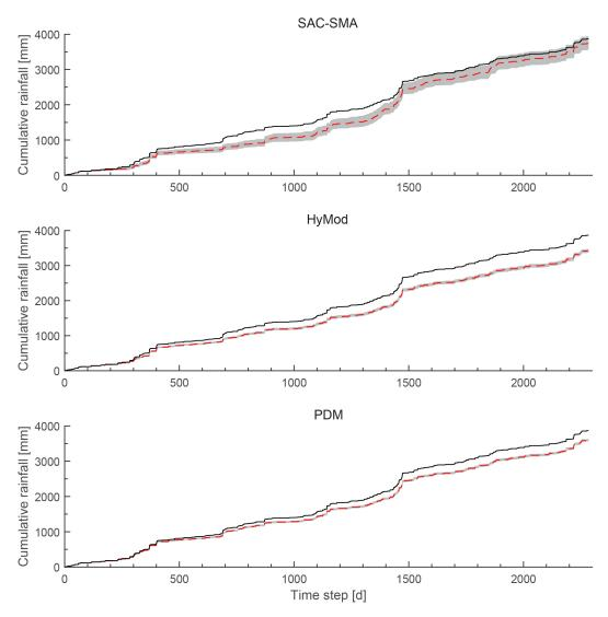
FIGURE 5.6: Cumulative rainfall series for the Warwick catchment. Observed rainfall is plotted using the black line while the mean and  $5^{th}$  to  $95^{th}$  percentile rainfall estimates were represented by the dashed red line and grey shading respectively.
