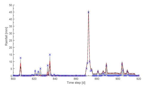
FIGURE 4.4: Rainfall estimates for experiment 3 over a 120 day period. The blue crosses and red line represent the observed rainfall and mean rainfall estimates, respectively. The dashed red line is the MAP rainfall estimate while the grey shading indicates the 5th and 95th percentile rainfall estimates.
