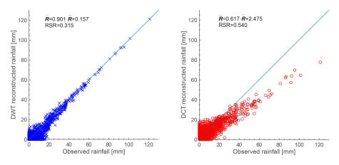
FIGURE 3.7: Comparison of the reconstructed DCT and DWT signal for the Leaf River (Collins) catchment using 20 POP.
