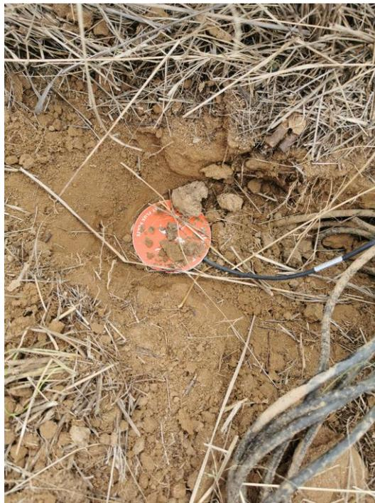
Figure 3: Replacement of 5cm Heat flux plate
