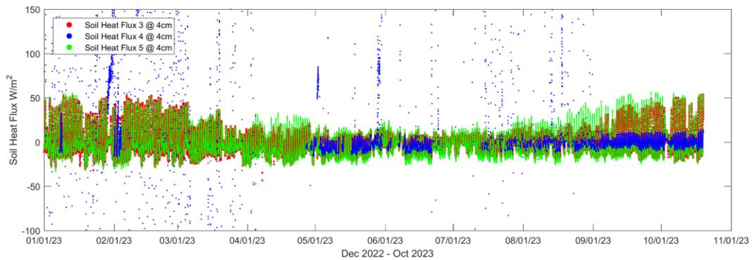
Figure 13: Soil Heat Flux at 4cm depth for 2023.
