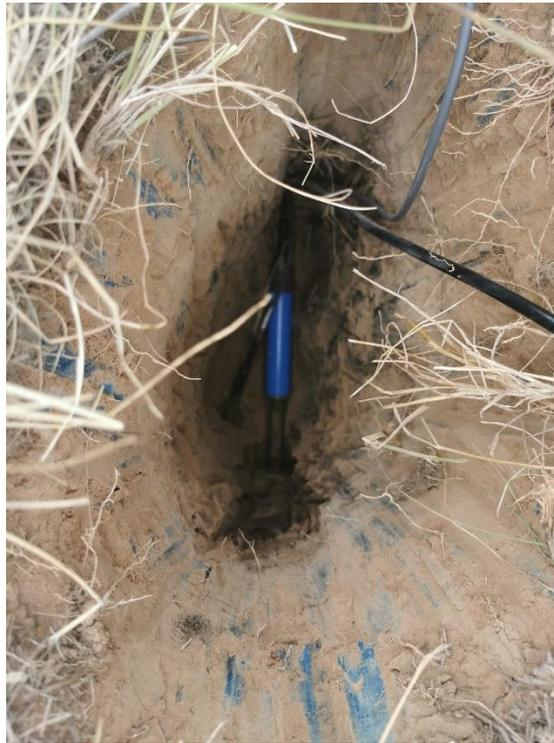
Figure 4: Replacement of 75cm Trime Pico soil moisture sensor.
