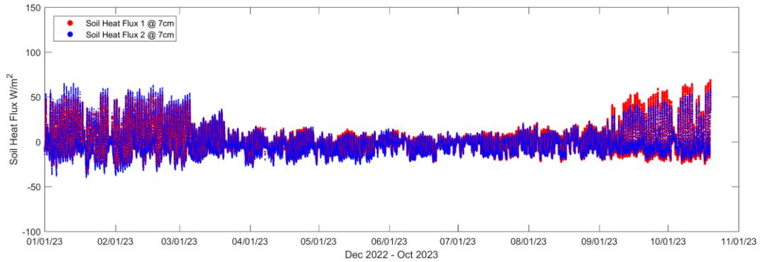
Figure 12: Soil Heat Flux at 7cm depth for 2023.
