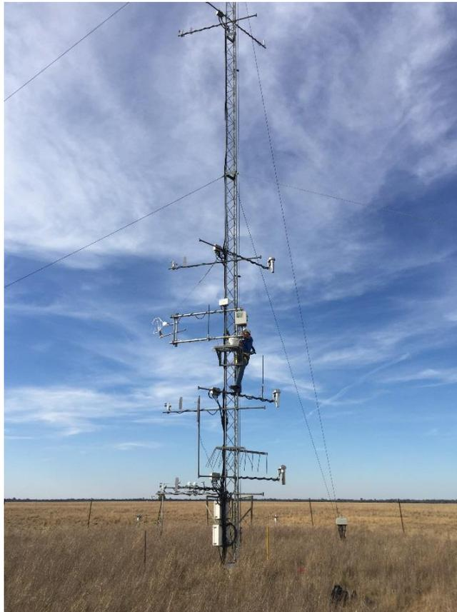
Figure 4: Monash technician climbing the tower to remove sensor for calibration.
