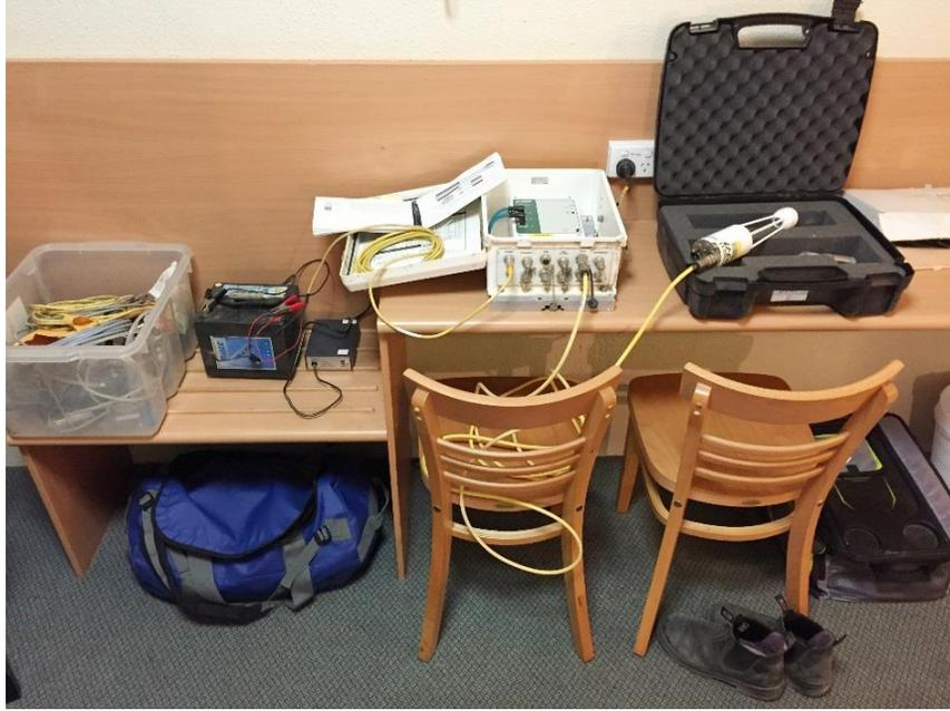
Figure 3: Calibration of the Open Path CO<sub>2</sub>/H<sub>2</sub>O Gas Analyzer (LI-7500A).
