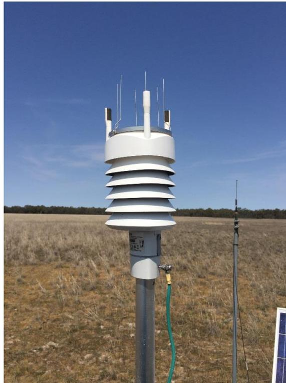
Figure 7: Mislocated Humidity and Temperature Probe (HMP 155) inside the Vaisala Weather Transmitter (WXT530), to be re-installed on to the tower at 16m height.
