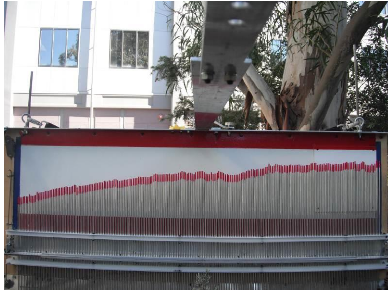
Figure 6-3. Pin profiler for surface roughness measurements.
