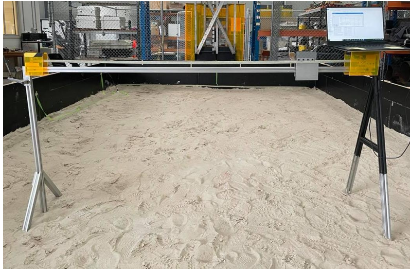
Figure 6-4. Pin profiler for surface roughness measurements.
