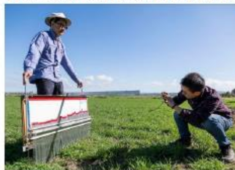
Fig. 4: Surface roughness sampling using a pin board profiler.
