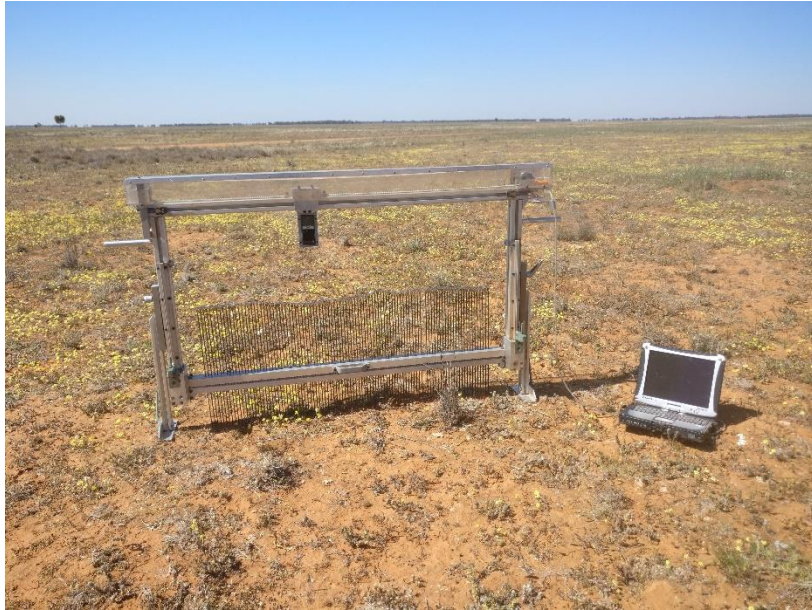
Figure 6-5. Laser-pin profiler for surface roughness measurements.
