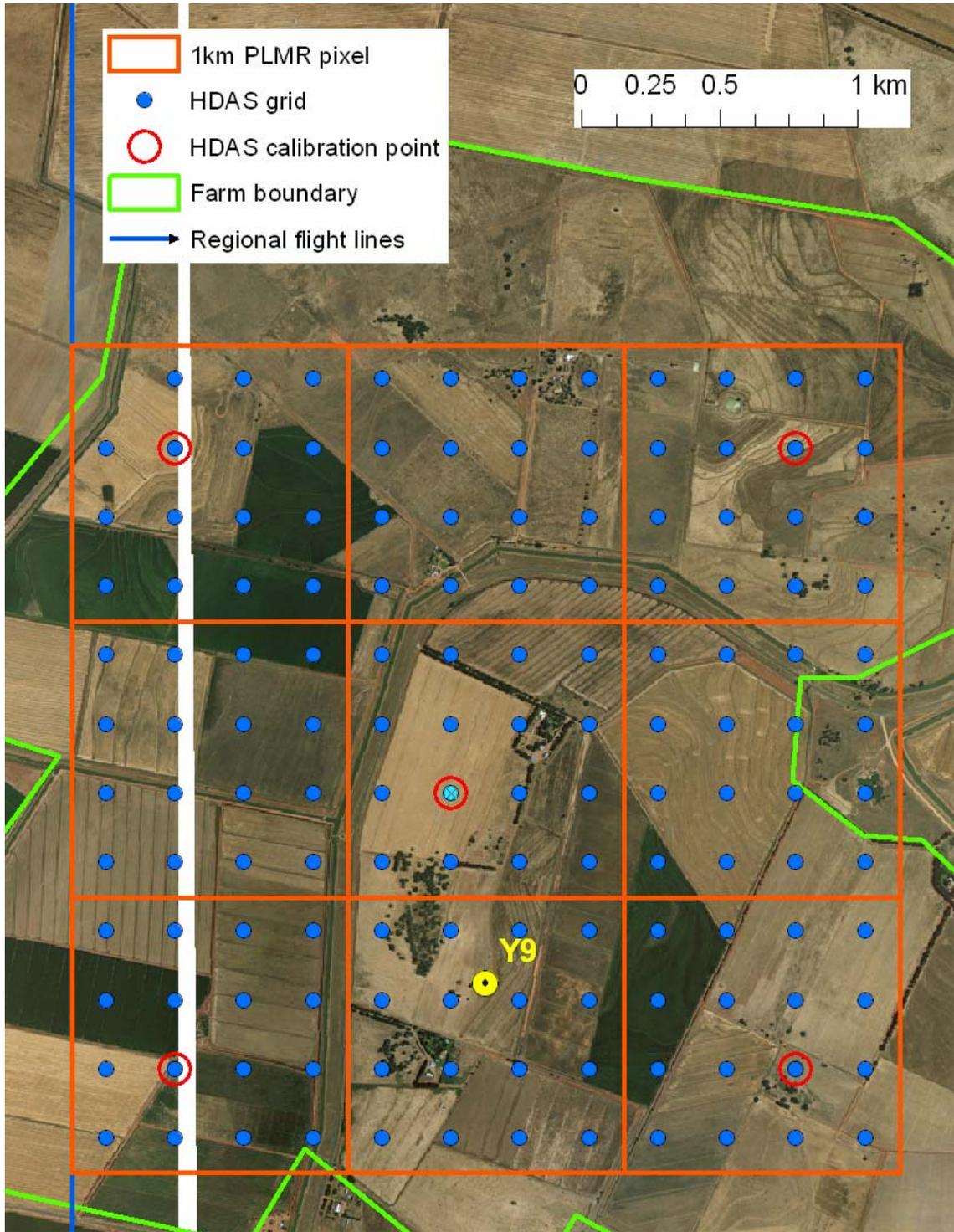
Fig. 5.5. Map of the soil moisture sampling grid in Yammacona.
