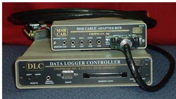
**Fig. B1.** Data logger controller & cable adapter box.
