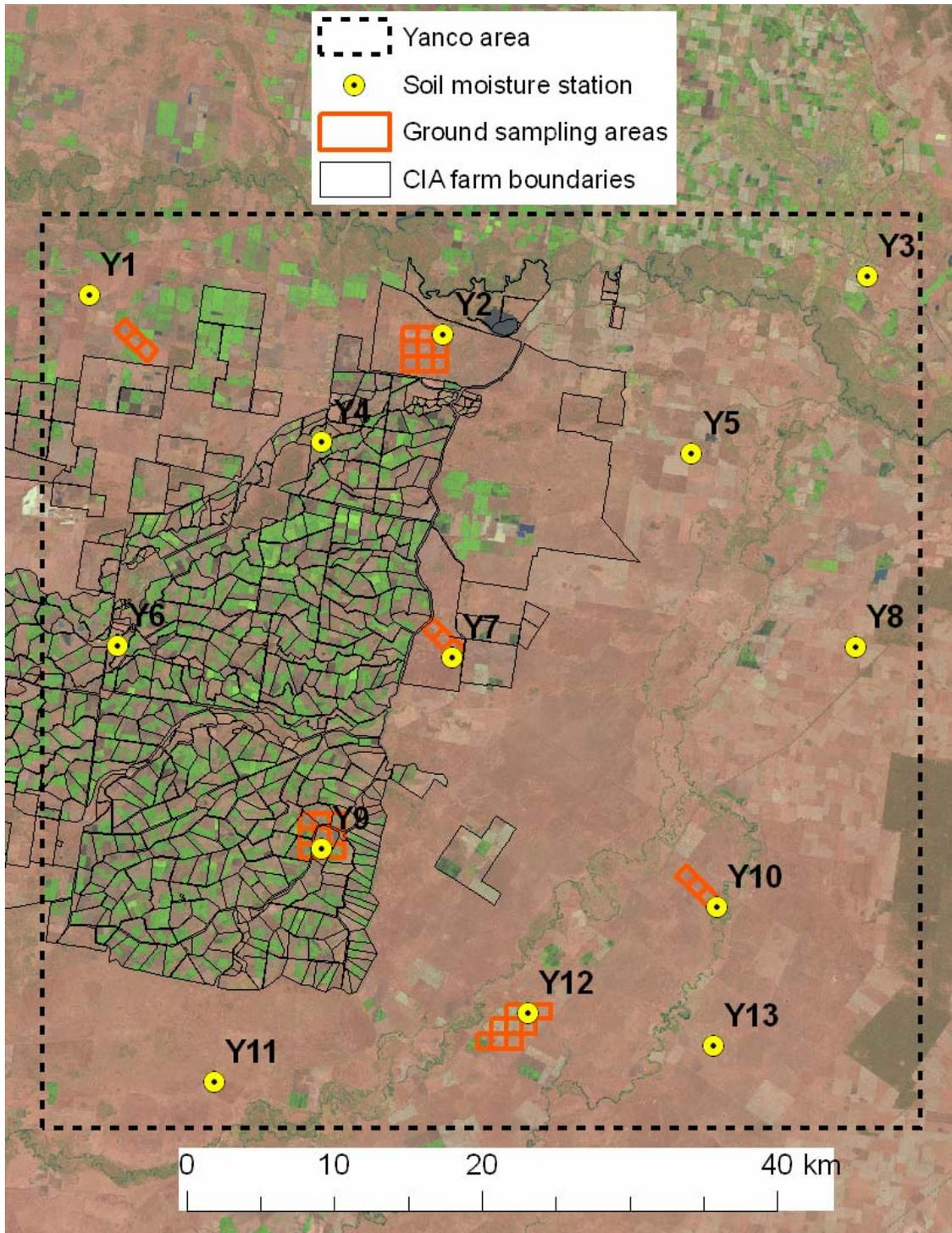
**Fig. 4.6.** The Yanco site is a 60km box with approximately one third of irrigated area (Coleambally Irrigation Area). The six ground sampling areas of NAFE'06 are indicated.
