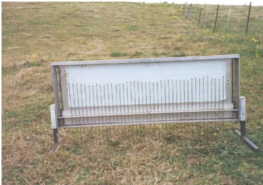
**Fig. 7.1.** Pin profiler for surface roughness measurements
