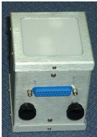
**Fig. 7.2.** CROPSCAN Multispectral Radiometer (MSR). (Size is 8 X 8 X 10 cm).
