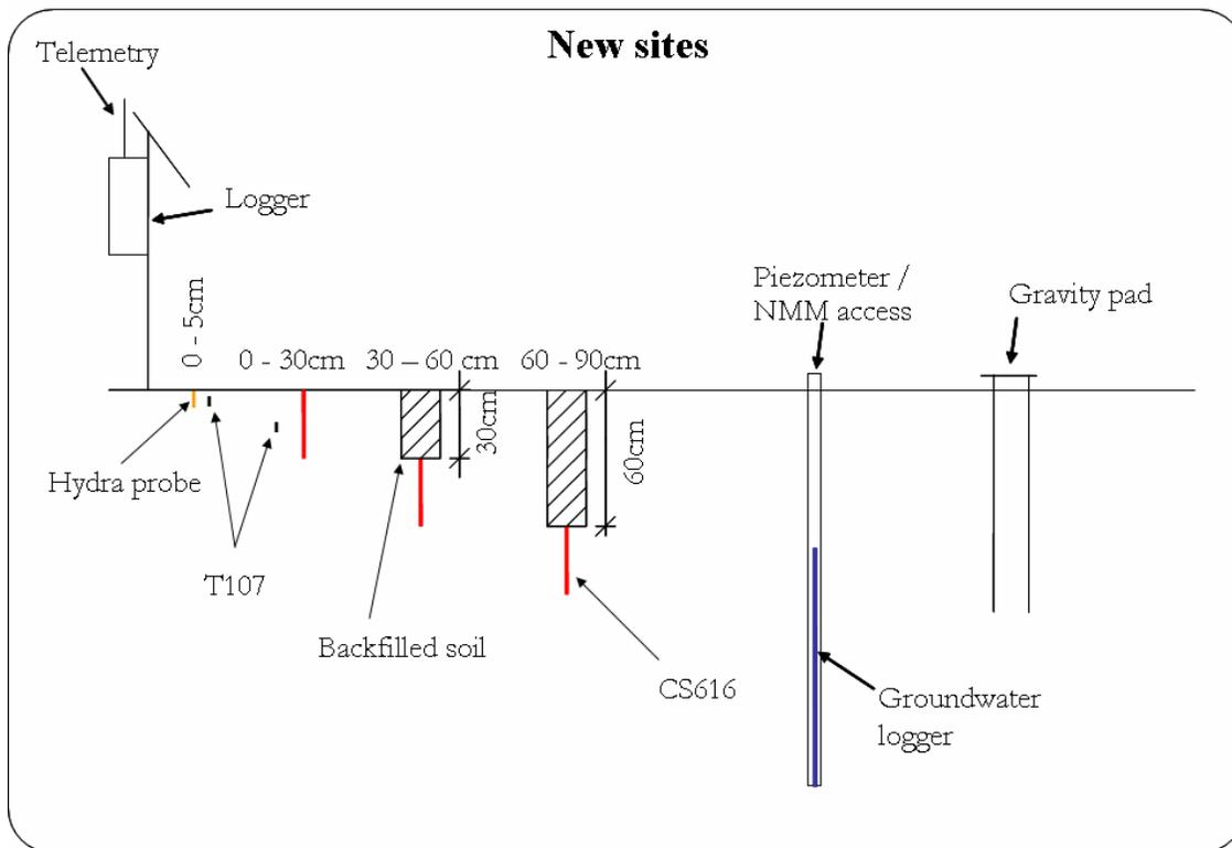
**Fig. 4.4.** Typical equipment at the original (2001) and new (2004) soil moisture sites in the Murrumbidgee catchment. Each site provides continuous data of rainfall, soil moisture at 0-5cm (or 0-7cm), 0-30cm, 30-60cm and 60-90cm and soil temperature and accommodates periodic measurements of gravity, groundwater and TDR soil moisture measurements.
