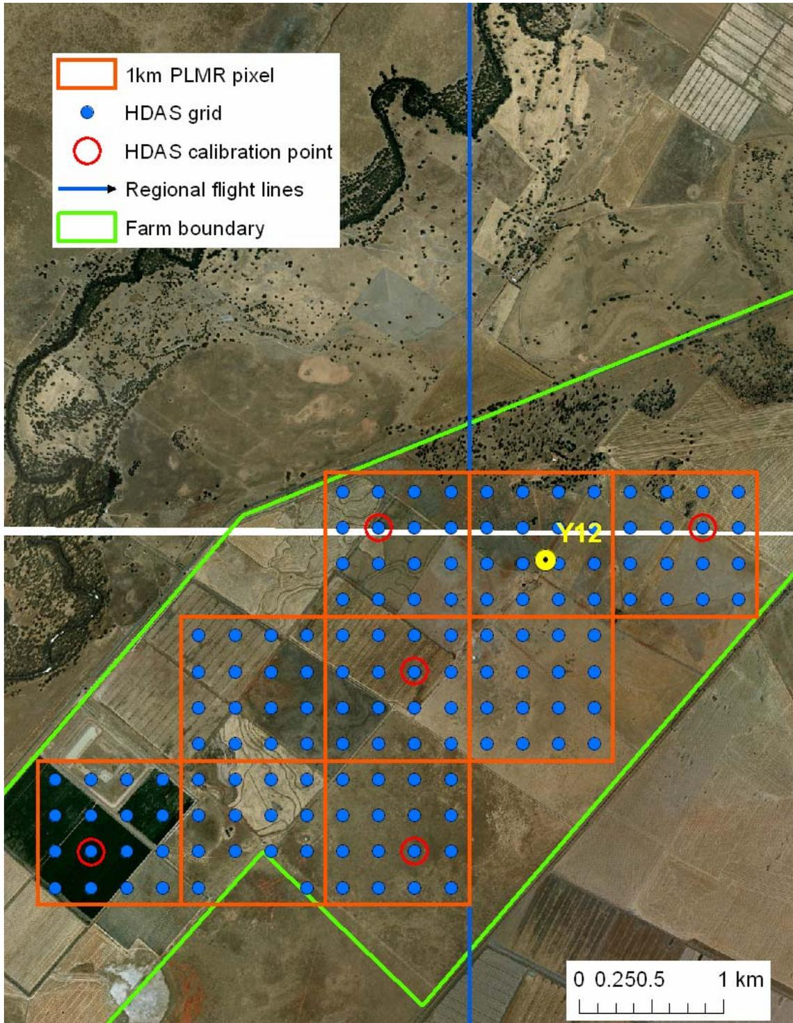
Fig. 5.6. Map the soil moisture sampling grid in Spring Bank.
