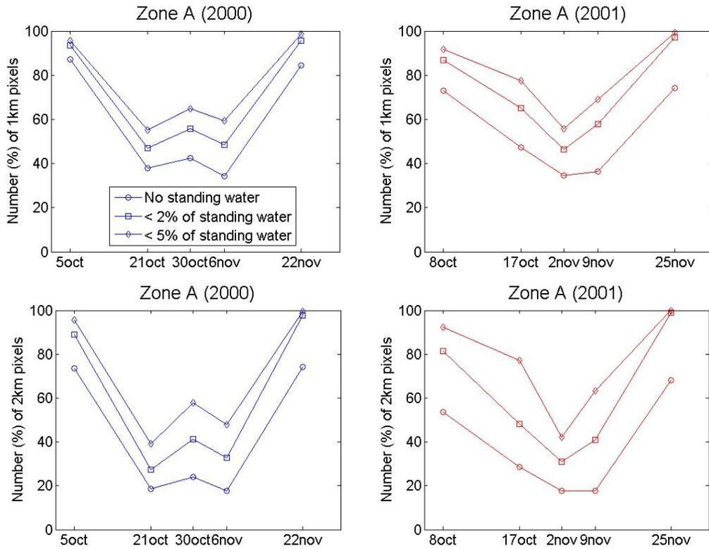
**Fig. 4.9.** Percentage of the 1-km and the 2-km pixels affected by 0, less than 2% and less than 5% of standing water in Zone A for 2000 and 2001.
