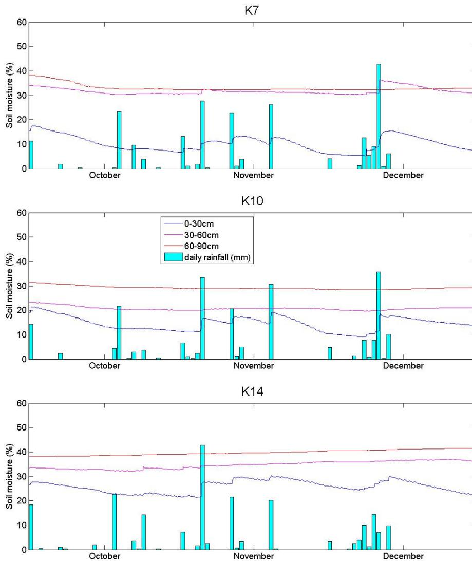
**Fig. 4.17.** Typical data collected continuously by the network of 14 soil moisture stations in the Kyeamba catchment in 2005.
