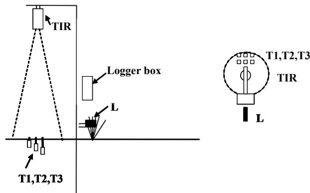
**Fig. 5.2.** Typical set up of the supplementary monitoring site (side view and top view); showing 1 cm (T1), 2.5 cm (T2) and 4cm (T3) soil temperatures; Thermal infrared (TIR) and leaf wetness (L) sensors.
