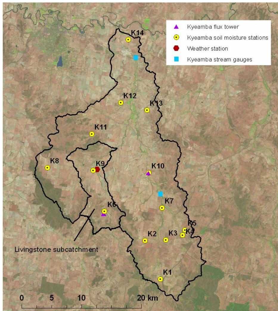
**Fig. 4.13.** The Kyeamba Creek catchment is currently equipped with 14 soil moisture stations, a 3D Eddy correlation flux tower (K10), and two stream gauges. Ground sampling will take place in the Livingstone Creek subcatchment, which includes a weather station (K9) and a Bowen ratio (K6).
