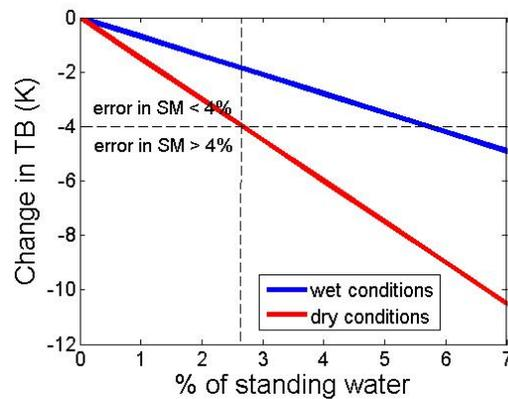
**Fig. 4.7.** Effect of standing water on PLMR data estimated with a brightness temperature (TB) of water of 110K and a TB of emerged land of 180K (wet conditions) or 260K (dry conditions).
