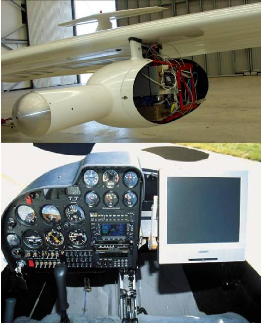
**Fig. 2.2.** View of one of the underwing pods with the cover off, and view of the cockpit showing cockpit computer display.
