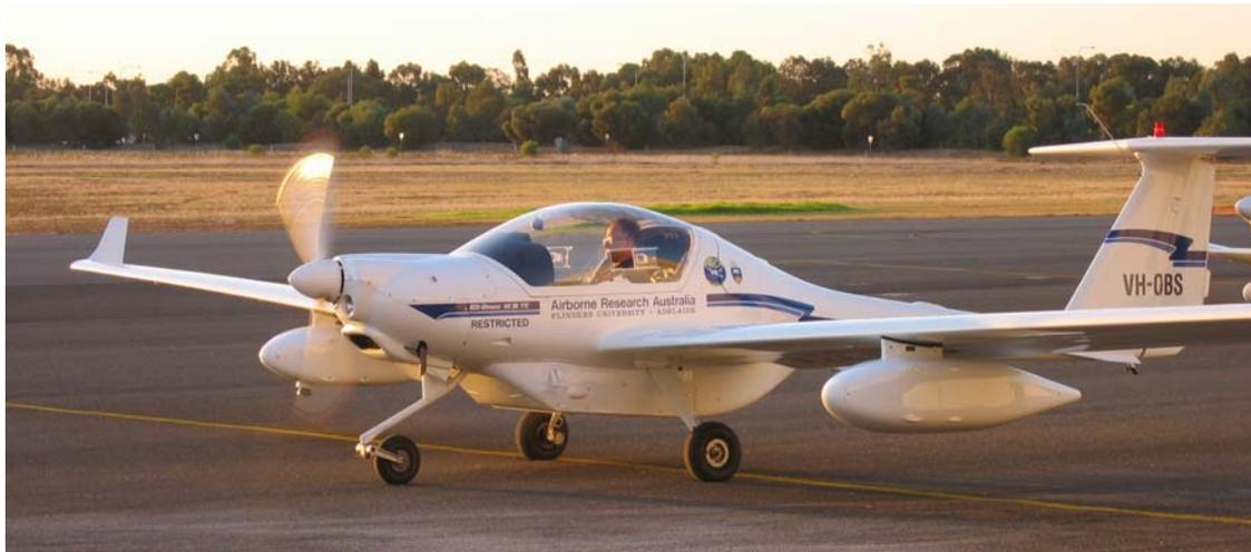
**Fig. 2.1.** The Diamond ECO-Dimona aircraft with PLMR mounted under the fuselage, and thermal imager, digital camera and NDVI scanner in an underwing pod.
