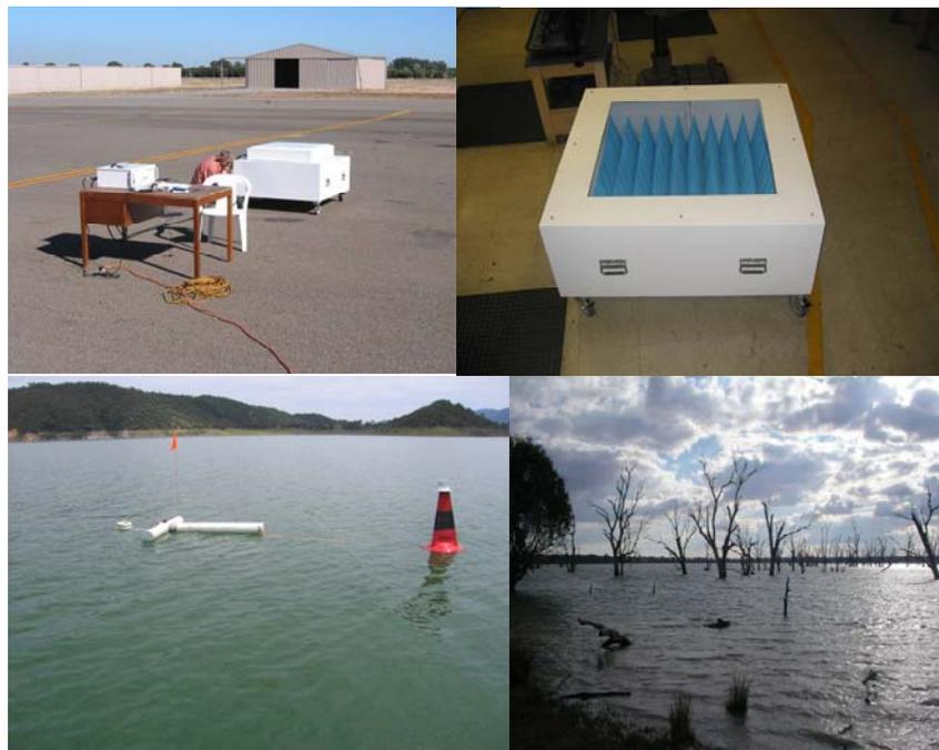
**Fig. 6.6.** Upper left: undertaking a sky cold point calibration with PLMR; upper right: the calibration box used for warm point calibration; downer left: the buoy used to monitor water temperature and salinity on the lake Tombullen; downer right: view of the Tombullen water storage from the bank.
