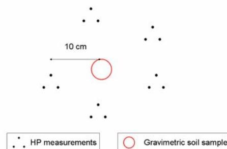
**Fig. 5.10.** A minimum of 3 HP measurements should be made in a radius of 10 cm around the soil sample.
