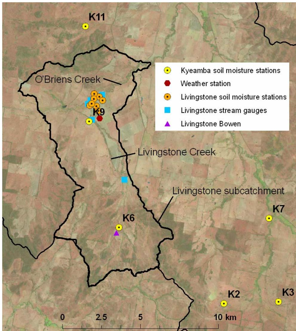
**Fig. 4.18.** The Livingstone Creek is a subcatchment of Kyeamba. In addition to the 2 soil moisture stations of the Kyeamba network, Livingstone is equipped with 8 supplementary soil moisture stations, 7 stream gauges and 1 Bowen ratio.
