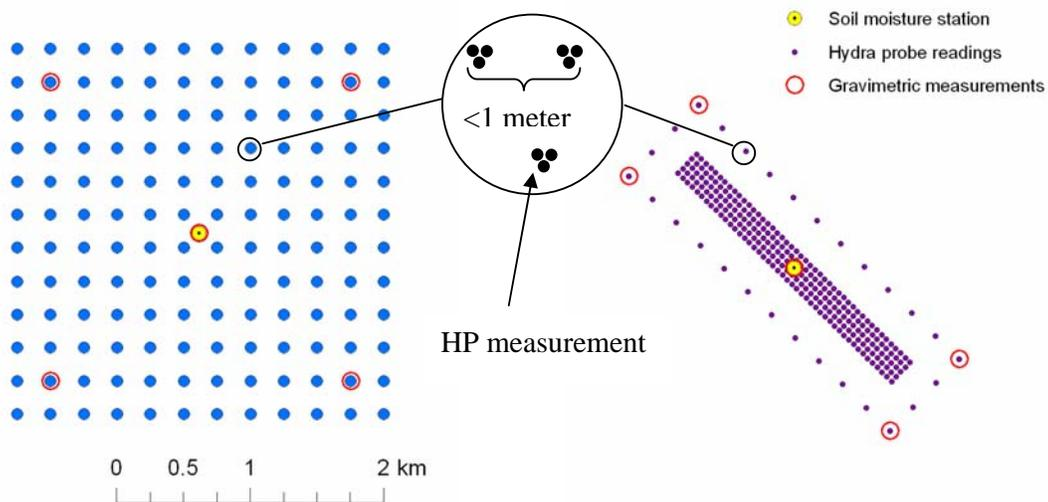
**Fig. 5.3.** Rationale of the soil moisture sampling during regional (left) and transect (right) days. Three HP measurements are to be made at each sampling point of the 50m and 250m grids.
