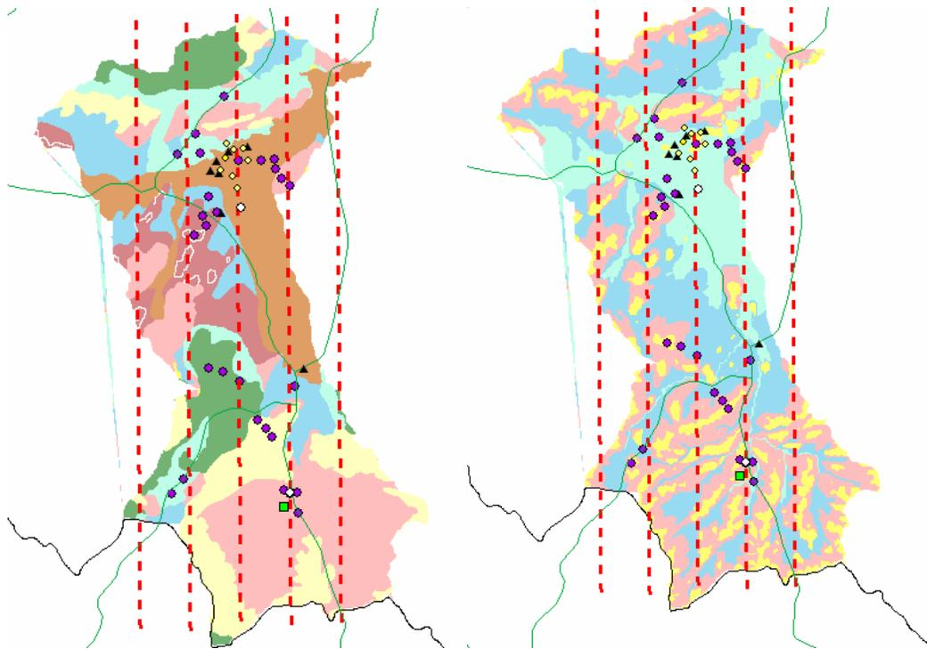
**Fig. 5.13.** Major soil texture types (left) and landforms (right) of the Livingstone Creek catchment. Yellow dots are existing soil moisture monitoring. Black triangles are stream gauging stations. White dots are weather stations. Green square is a Bowen Ratio. Purple dots are the proposed manual soil moisture field data collection sites. The medium-resolution flight lines are also shown.
