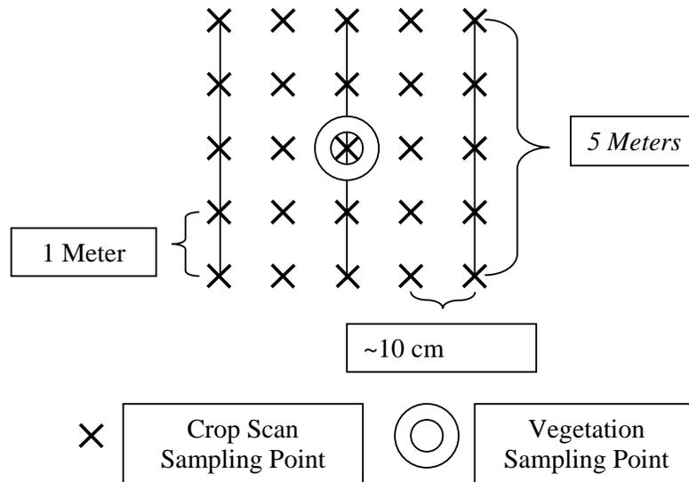
**Fig. 7.3.** Illustration of the surface reflectance protocol.
