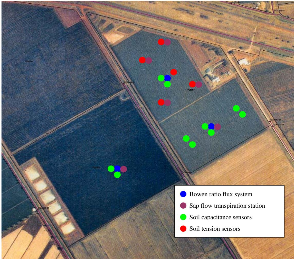
**Fig. 4.21.** Location of the Bowen ratio flux systems, sap flow stations, and soil capacitance/tension sensors in the two vineyard blocks.
