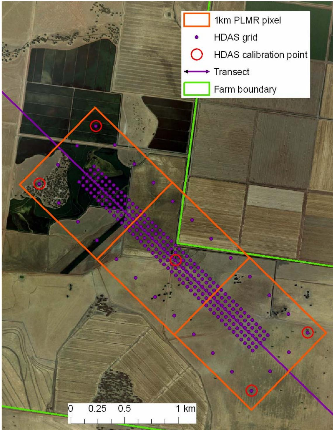
**Fig. 5.7.** Map of the soil moisture sampling grid in Uri Park (Y1). Note that the monitoring station is off to the top left.
