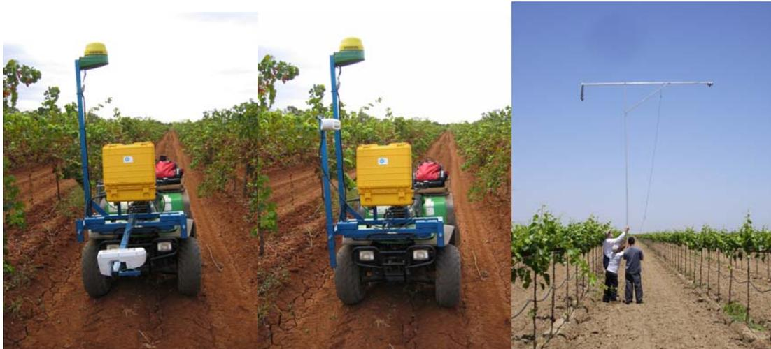
**Fig. 5.16** The NDVI and TIR sensors are mounted on a quad bike. On the right, using a ceptometer.
