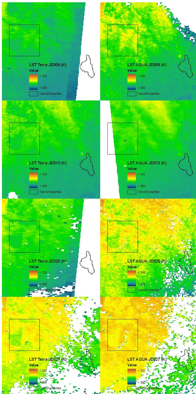
**Fig. 3.1.** Example of MODIS surface temperature images acquired in November 2005 over the study area of NAFE'06. On Julian days 309, 313, 325 and 327, MODIS images were acquired at approximately 10am on board Terra (left) and 2pm on board AQUA (right).
