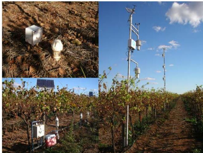
**Fig. 4.20.** Soil moisture sensors in the upper left, sap flow sensors in the lower left and the 3 Bowen ratios on the right.
