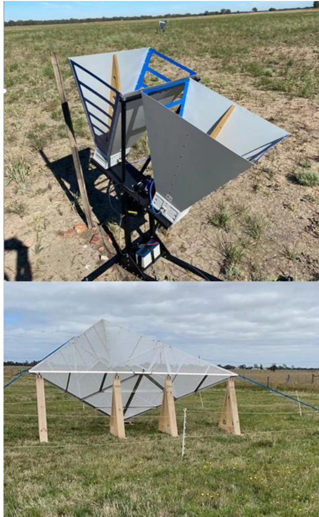
Figure 4-6. Polarimetric Active Radar Calibrators (top) and Passive Radar Calibrator (bottom).
