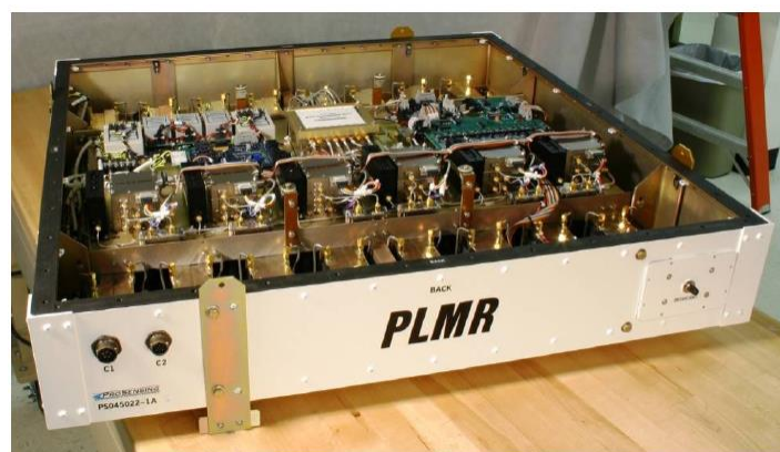
Figure 2-3. View of PLMR with the cover off.
