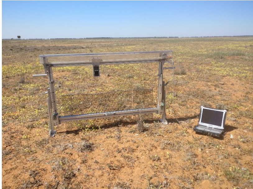
Figure 6-5. Laser-pin profiler for surface roughness measurements.
