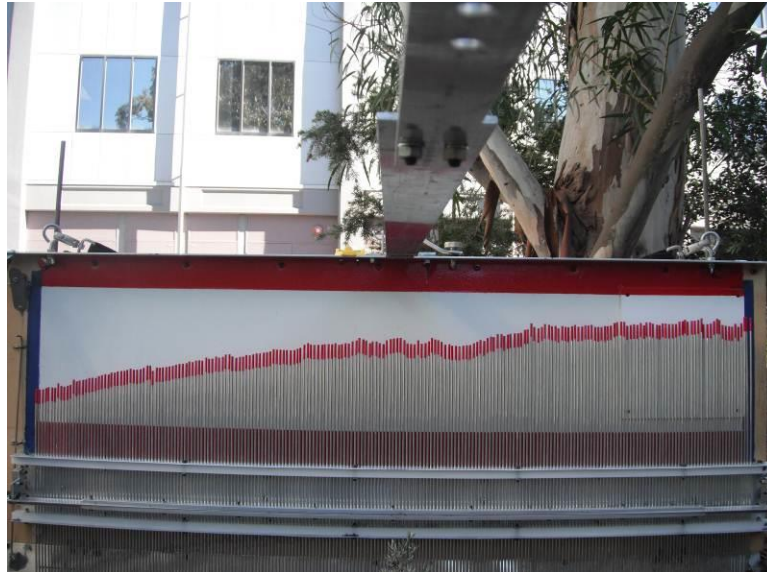
Figure 6-3. Pin profiler for surface roughness measurements.
