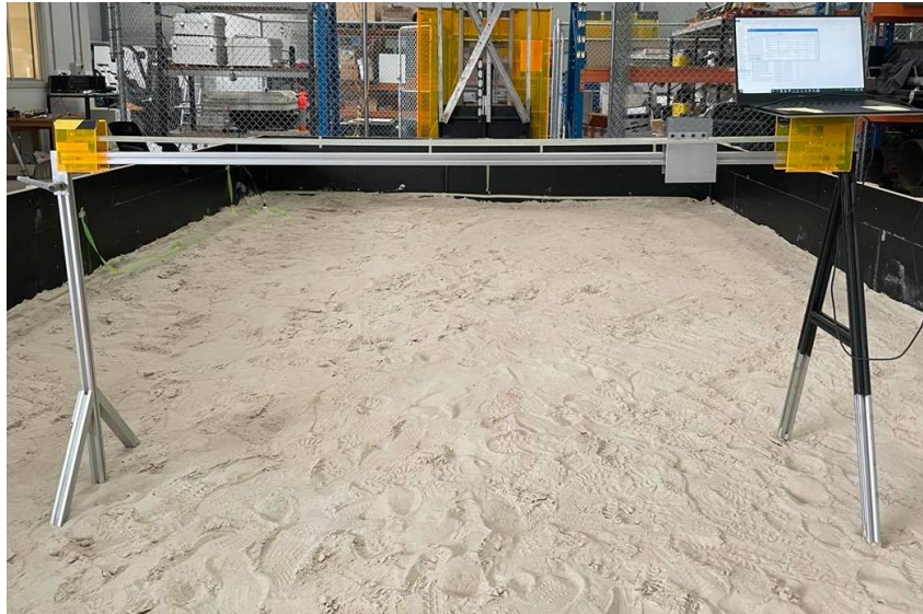
Figure 6-4. Laser profiler for surface roughness measurements.
