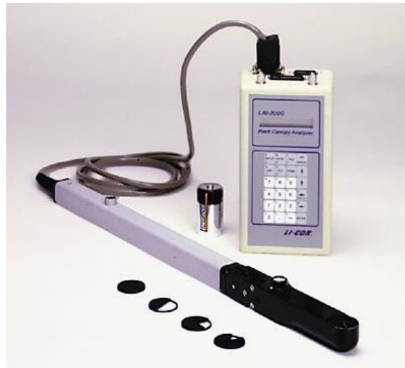
Figure 6-2. The LAI-2000 instrument.
