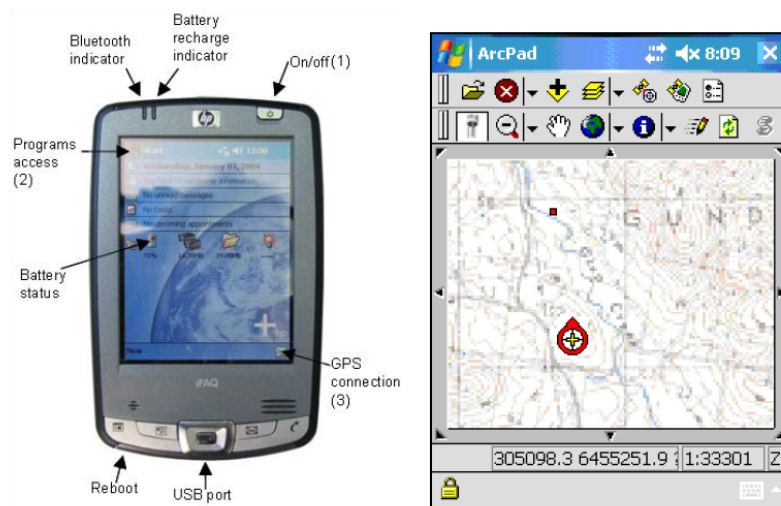
Figure 2. General layout of the iPAQ (left) and HDAS sampling screen (right).
