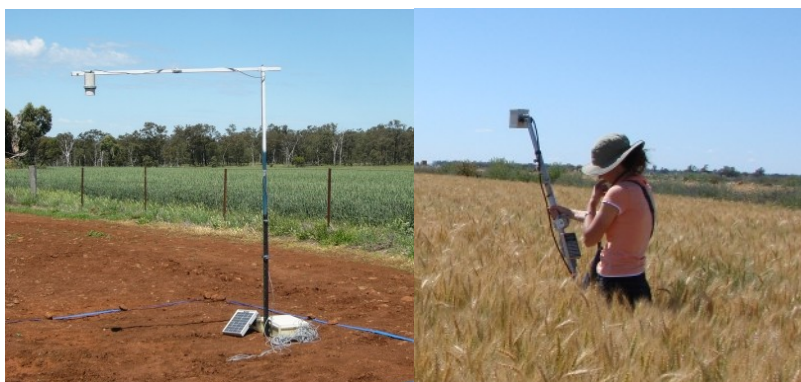
Fig. 4. Short term monitoring station with thermal infrared sensor observing the surface temperature (left) and non-destructive vegetation measurements with a CropScan (right).
