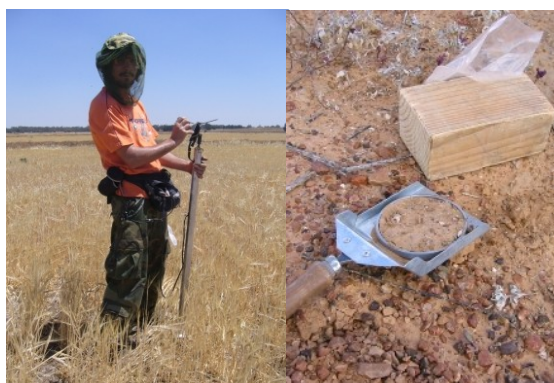
Fig. 3. Soil moisture probe and soil sampling example.
