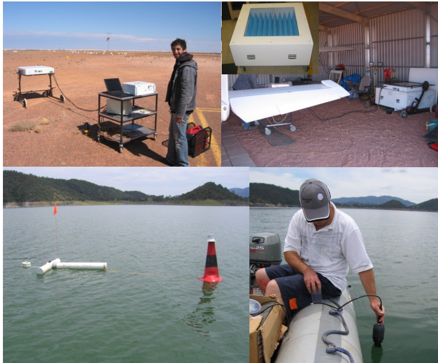
Figure 5-5: Upper left: undertaking a sky cold point calibration with PLMR; upper right: undertaking a warm point calibration with the calibration box shown in the inset; lower left: the buoy used to monitor water temperature and salinity; lower right: undertaking a boat transect of water salinity and temperature.
