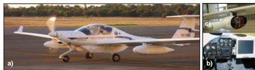
Fig 2: a) The Diamond ECO-Dimona Small Environmental Research Aircraft (SERA) platform, b) the cockpit with computer display of flight track and sensor output, and c) one of the two multipurpose instrument pods.
