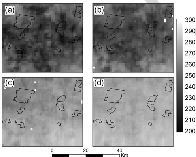
Fig. 6. PLMR L-band passive microwave H-polarized observations (K) for the four regional mapping flights. (a) October 31. (b) November 7. (c) November 14. (d) November 21. The boundaries of the eight focus farms for ground sampling are displayed for reference.
