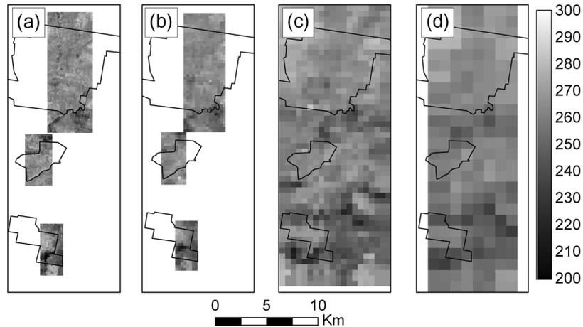
Fig. 7. Example of the multiresolution PLMR L-band H-polarized passive microwave observations (K) in the Krui area for November 1, 2005. Nominal resolutions displayed are (a) 62.5 m, (b) 250 m, (c) 500 m, and (d) 1000 m. The boundaries of the focus farms for ground sampling are displayed for reference.
