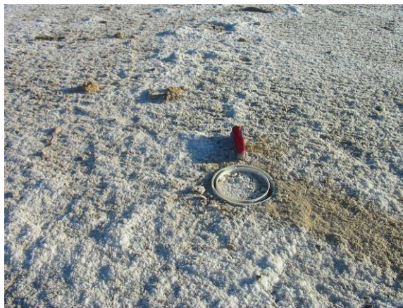
Figure 3 Microlysimeter installed in a salt scald coinciding with the Cadnaowie Formation and Bulldog Shale boundary, Neales catchment.
