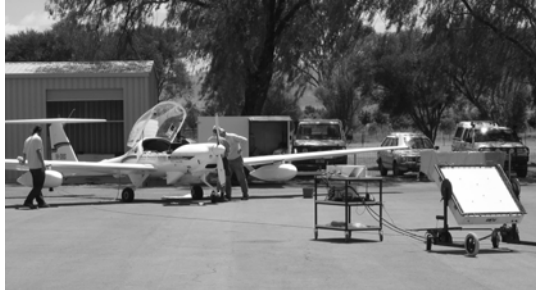
Figure 7. The Diamond ECO-Dimona aircraft showing bulkheads under the fuselage for mounting PLMR, with thermal imager, digital camera and tri-spectral scanner and lidar in an underwing pod. The foreground shows PLMR undergoing a sky calibration.
